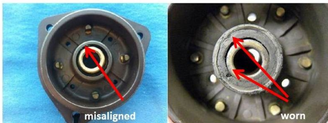
Figure 2: Two examples of unserviceable distributor blocks
