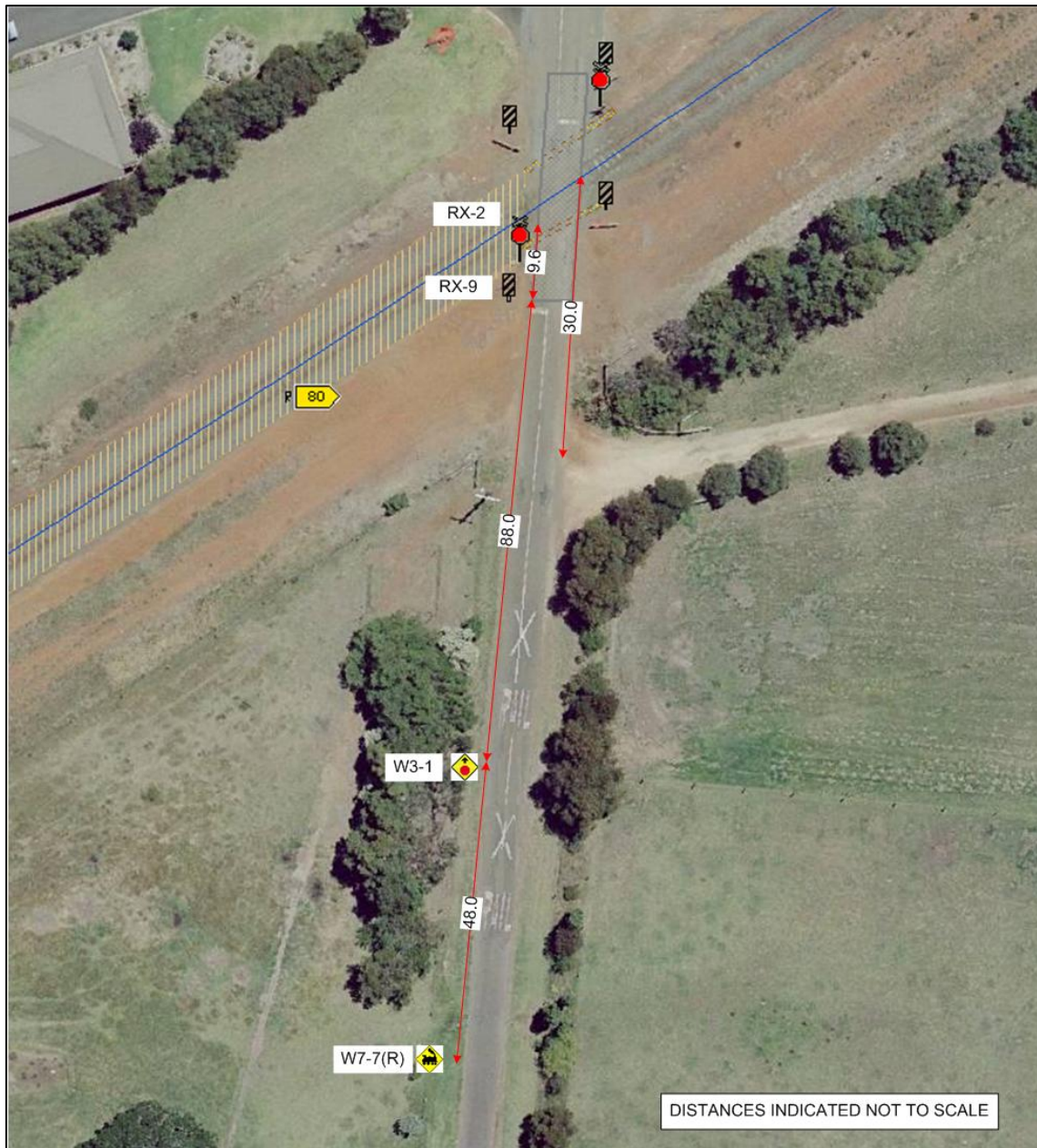
Figure 5: Signage and road markings on approach to Brown Street level crossing from south
