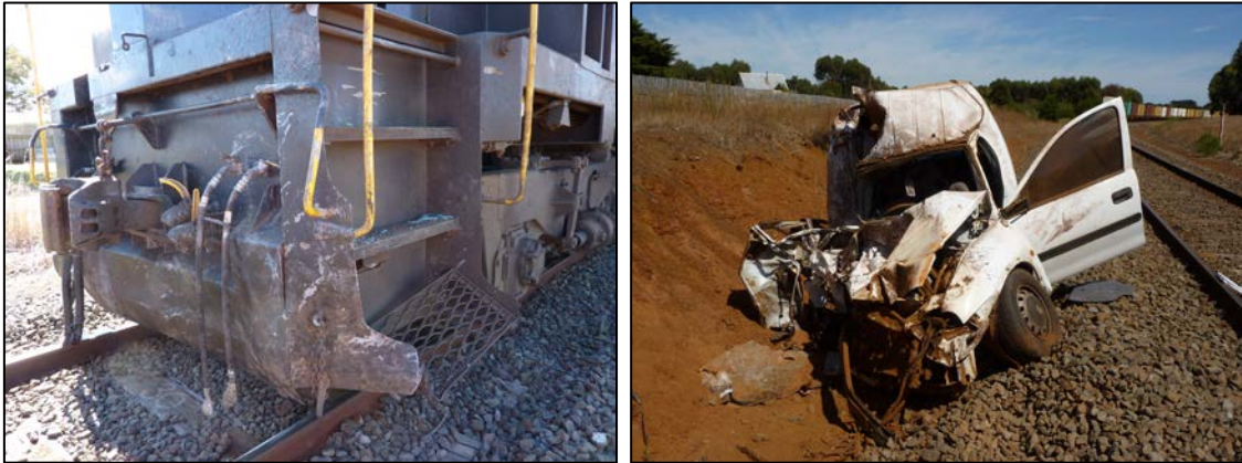
Figure 2: Damage to lead locomotive T378 and the motor vehicle
