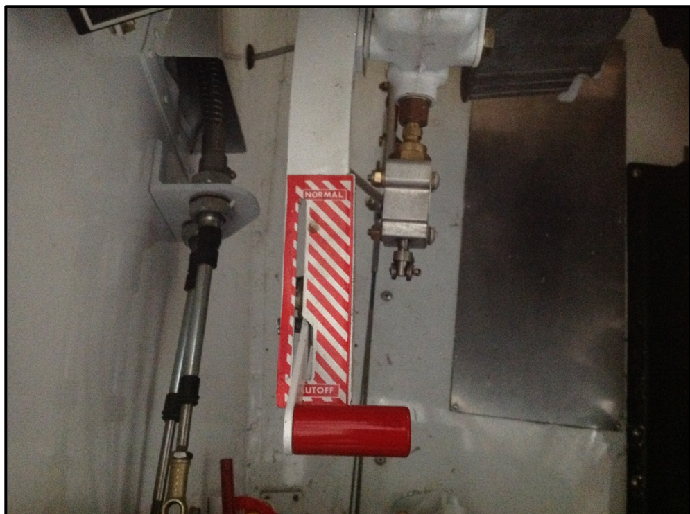
Figure 3: Emergency cut-off lever in the cut-off position (example aircraft)
