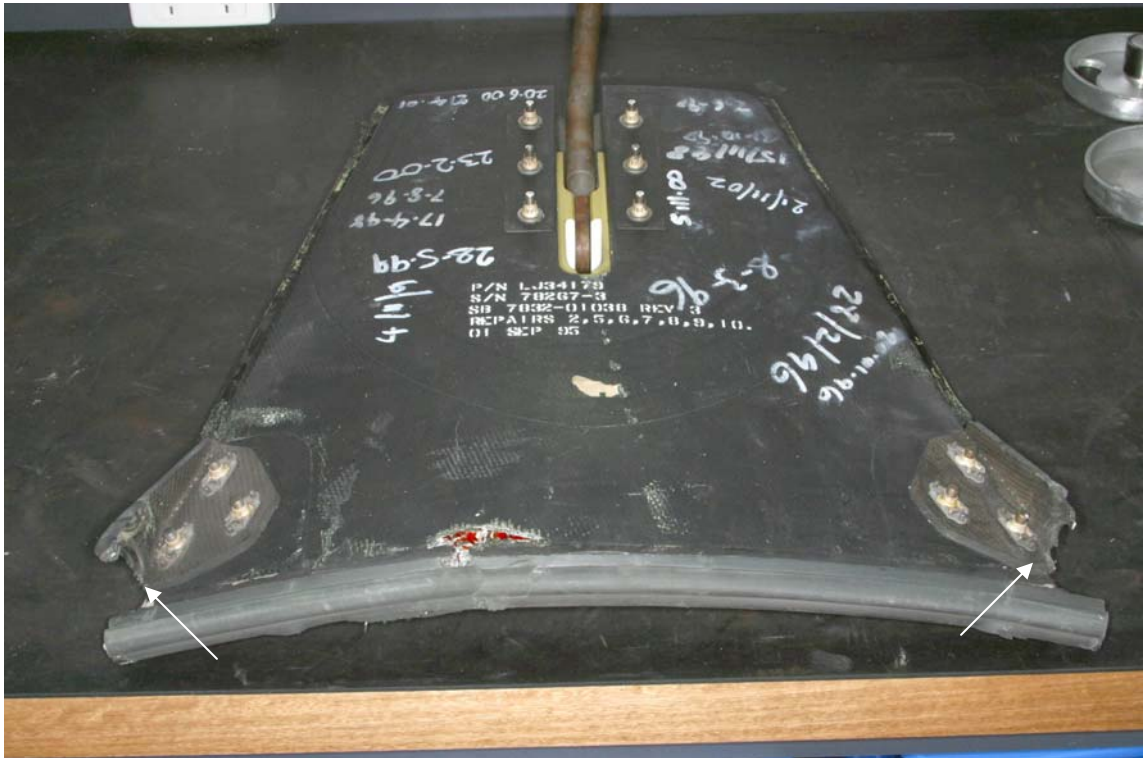
Figure 4. Thrust reverser blocker door showing failure of hinge points.
