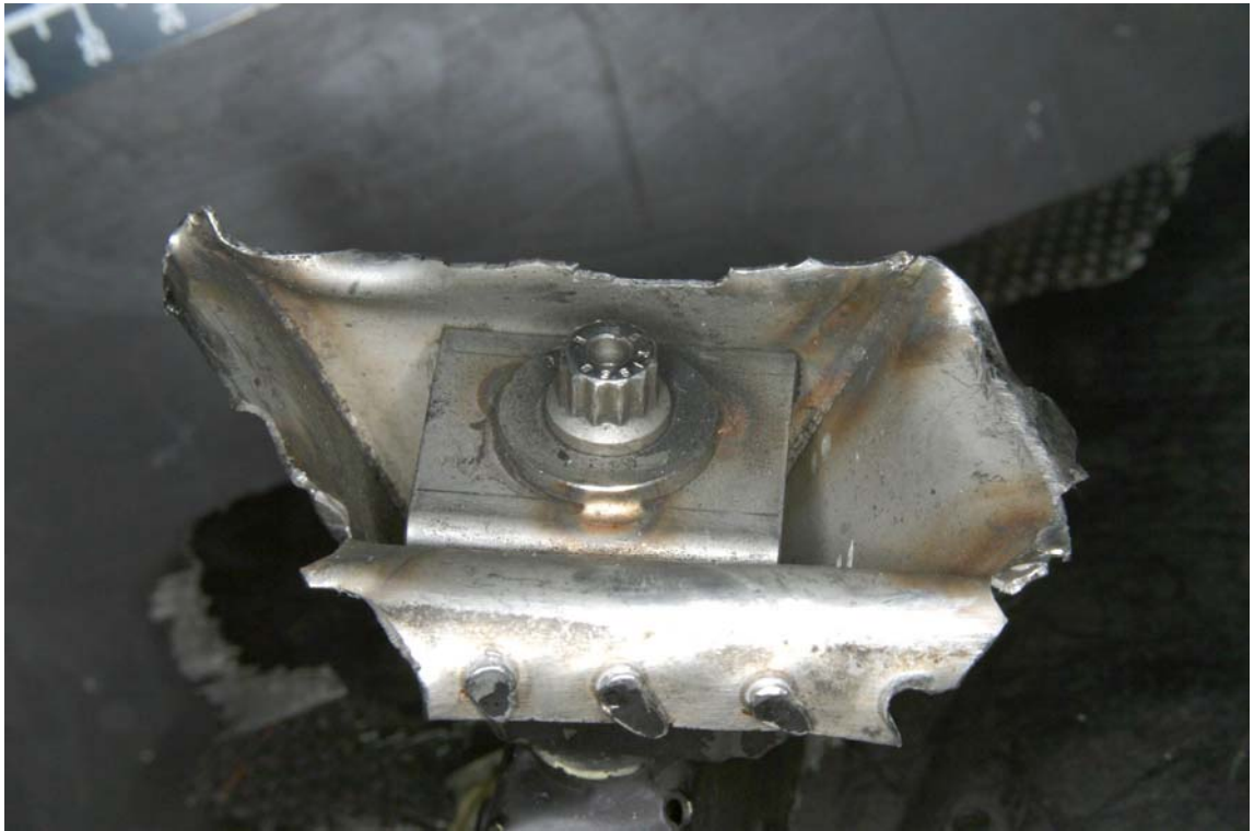
Figure 13. Base of the other bolt tower showing a combination of cracking around the flange transition and ductile tearing and pull-through of the riveted connection.
