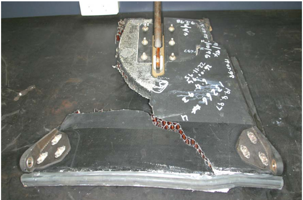
Figure 5. Blocker door major sections illustrating nature of break-up.
