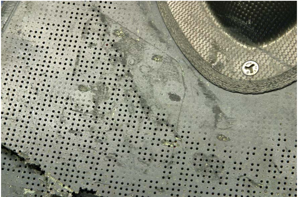
Figure 8. Close view of the impact mark shown in figure 7 above. Compare with figure 14 showing the drive fairing panel.
