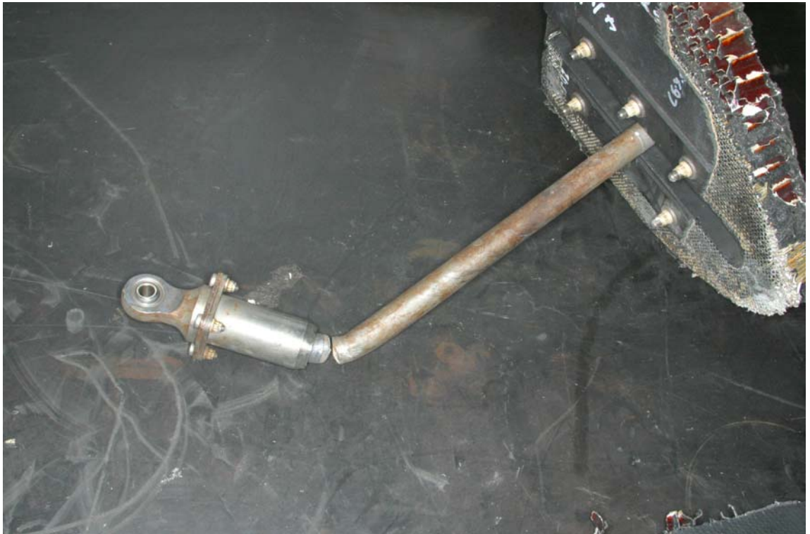
Figure 6. Blocker door actuator rod bending failure.
