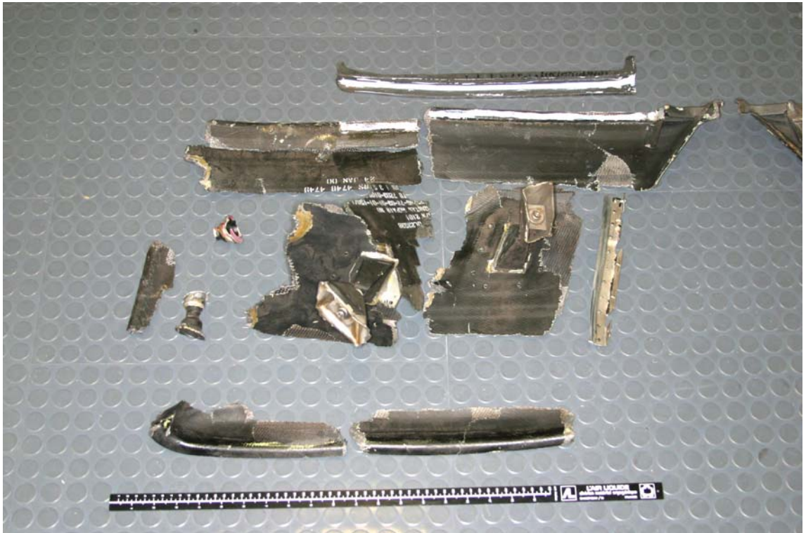
Figure 1. Received remnants of the INA drive fairing – side 1.
