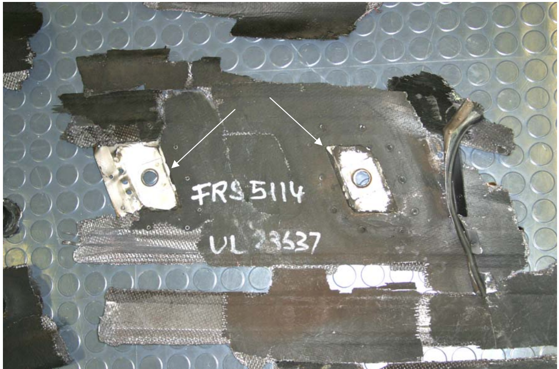
Figure 10. Inside surfaces of a drive fairing panel. Note the complete separation of the central bolt towers from their base panels.
