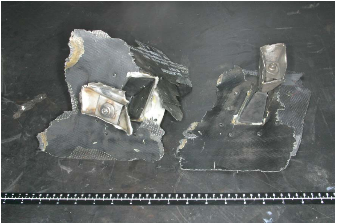
Figure 11. Separated drive fairing bolt towers.
