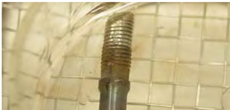
Figure 8. Bolt E being agitated in distilled water. Note the reddish solute being removed from the threaded section of the bolt.
