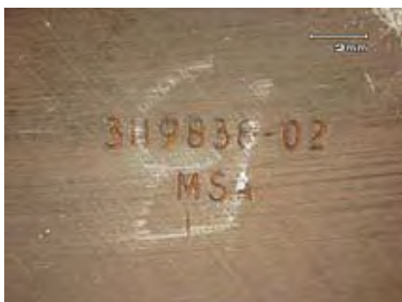
Figure 1. One of the turbine bolts from engine s/n 115120 head showing the part number on the bolt head.
