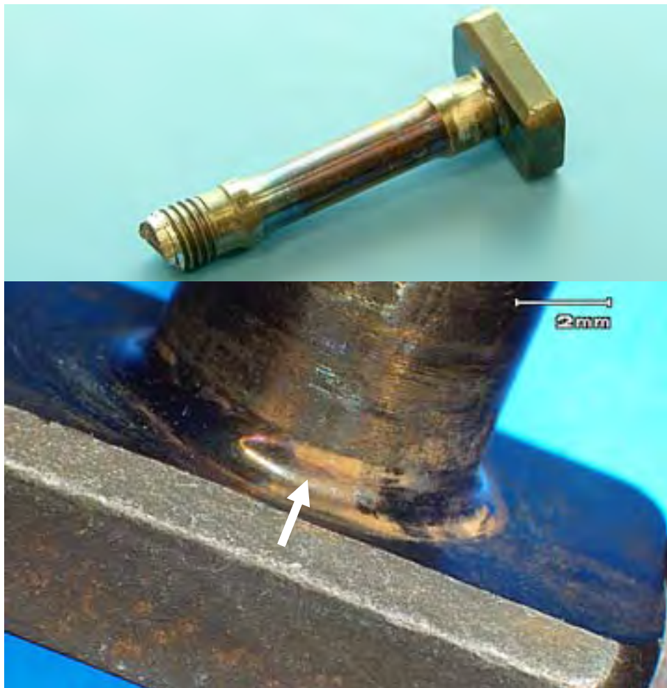
Figure 11(a). Extent of dust deposit in the bolt head fillet.
