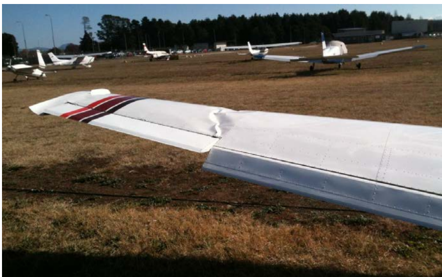
Figure 1: Left wing damage to VH-NFP
