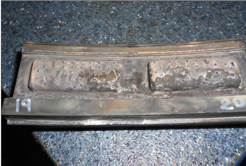
Figure 6: Dust accumulation in HPT stage-1 shroud hangers
