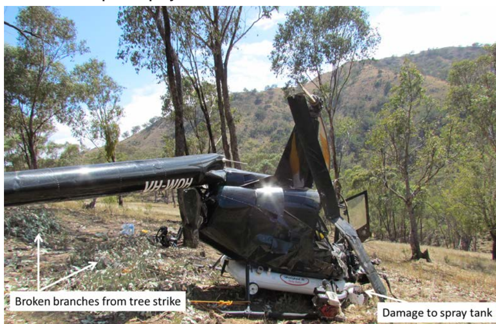
Figure 5: WOH (uprighted) showing the damage to the surrounding branches and helicopter's spray tank
