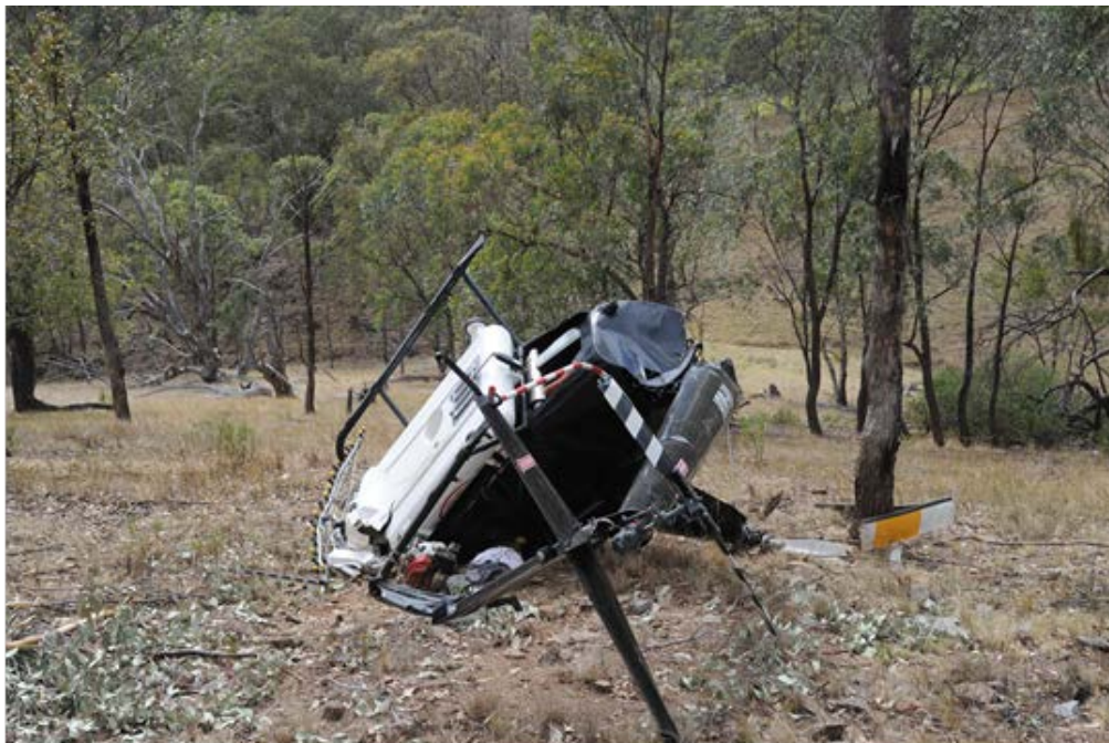
Figure 3: Accident site showing the helicopter's position at ground impact
