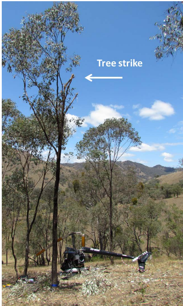
Figure 4: Tree strike and uprighted helicopter position, next to the ground impact point
