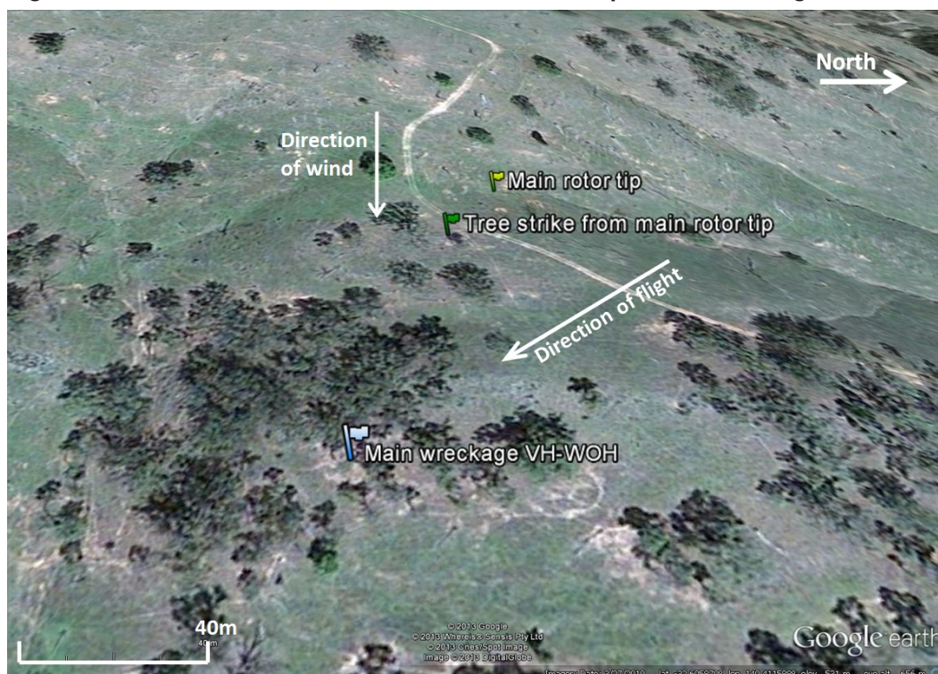
Figure 6: Location of the detached main rotor blade tip and tree damage
