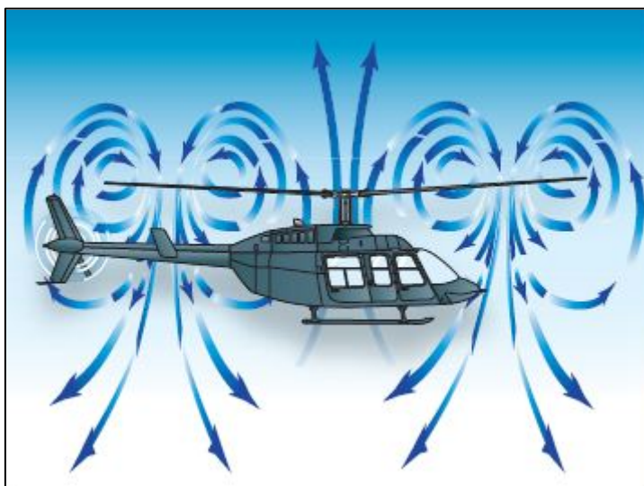
Figure 2: Vortex ring state
