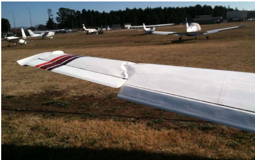
Figure 1: Left wing damage to VH-NFP
