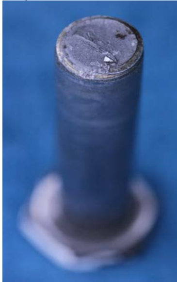
Figure 2: Failed lower torque link attachment bolt
