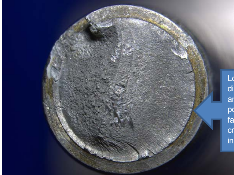
Figure 3: Bolt fracture surface
