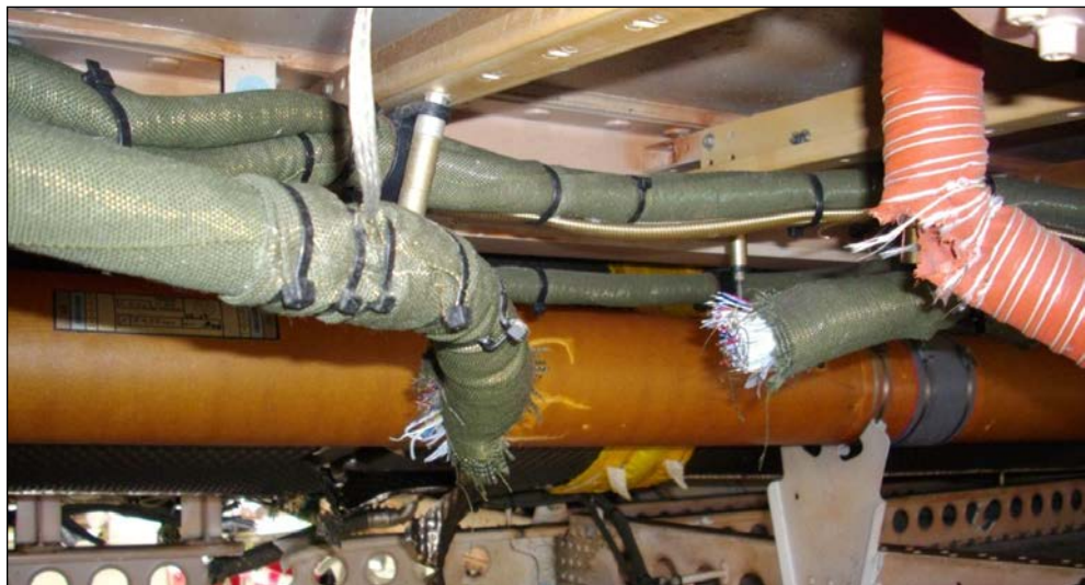
Figure 10: Damage to wiring in the belly fairing
