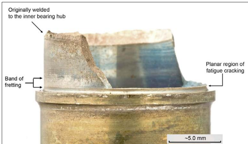
Figure 44: Oil feed stub pipe fretting
