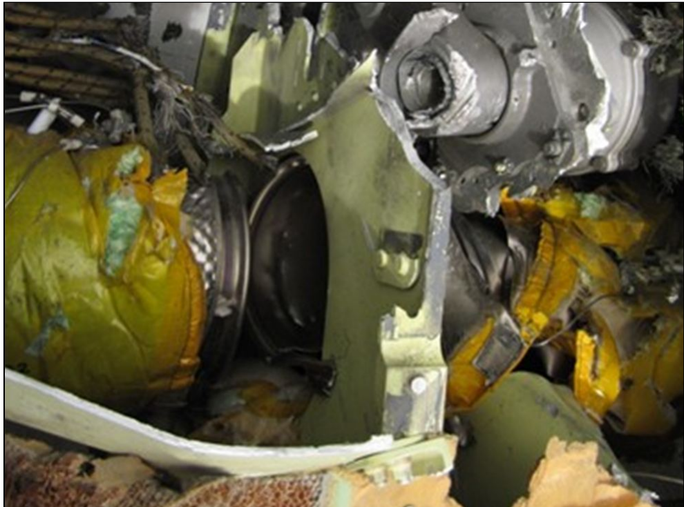
Figure 60: Bleed air duct damage
