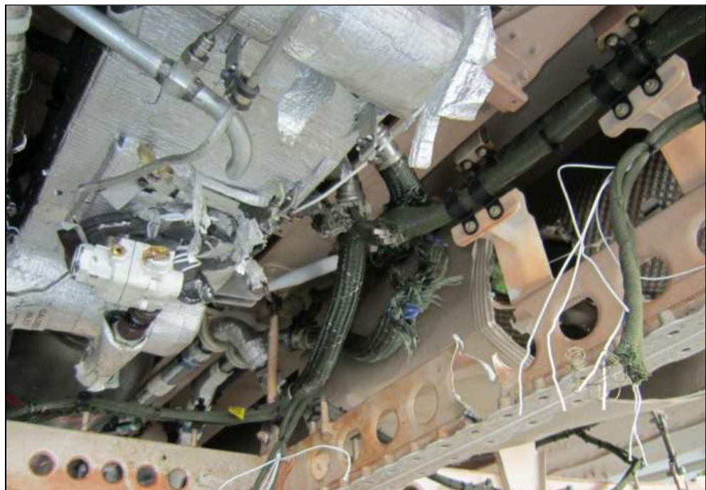
Figure B49: Wiring harnesses within the belly region of the aircraft structure were damaged from the liberated engine debris. Shown is harness 500HW1 (route 1PZ). All wires were severed
