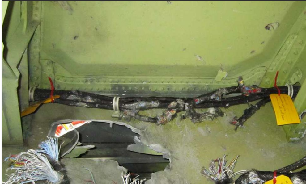
Figure B45: Detailed locations of damage to the 1G route (electrical harness 3029VB), primarily between Rib 9, 10 and 11 of the left wing; four of the 9 feeder and exciter cables have been severed—red framed area expanded in Figure B46
