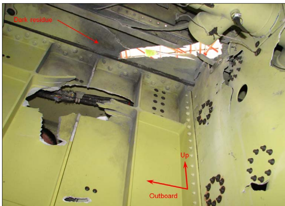
Figure 23: Dark residue in left inner wing fuel tank (looking up and forward)
