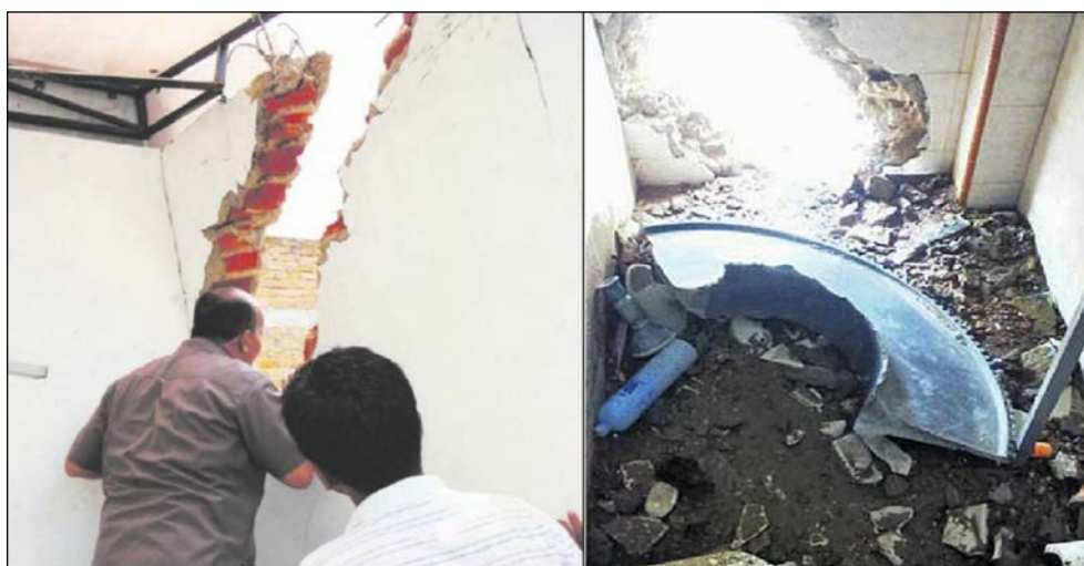
Figure 12: Property damage from a section of the No. 2 engine turbine disc
