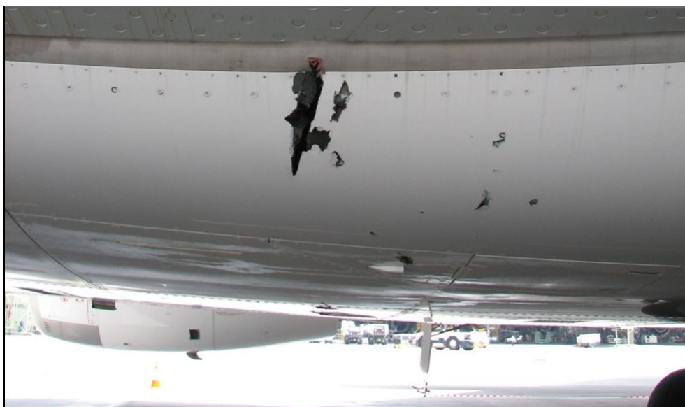
Figure B32: A smaller, high energy fragment of the IP turbine cut a swath directly through the belly fairing of the aircraft—view looking to the right of the aircraft with the No. 3 engine in the background.
