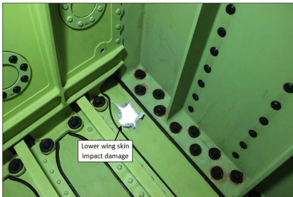
Figure B13: Impact damage to the lower wing skin
