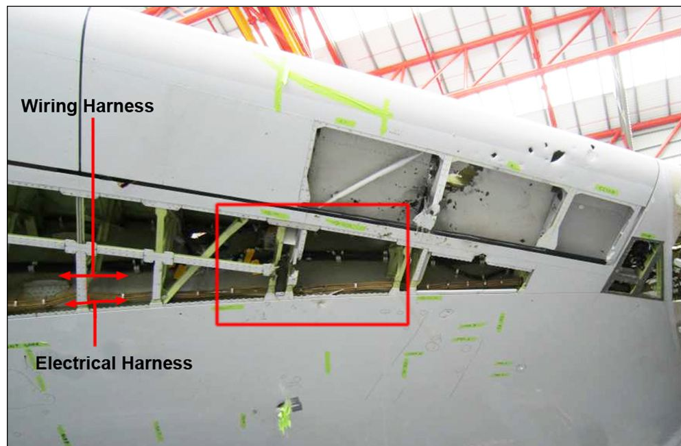
Figure B39: General location of the wiring harness damage within the leading edge of the left wing—red framed area expanded in Figure B40
