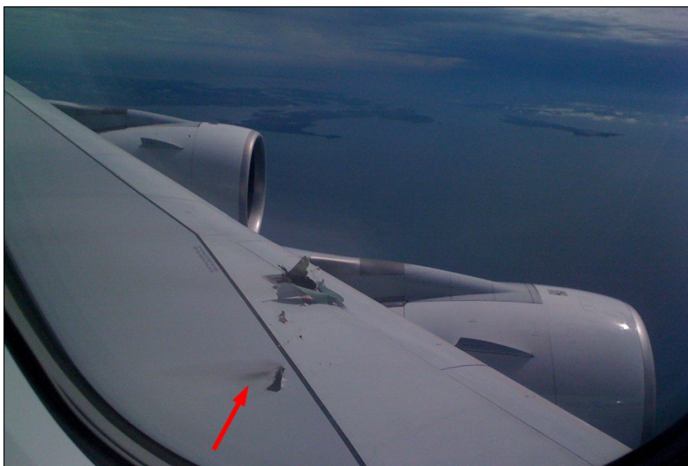
Figure D1: View from the window on the upper deck, left side showing the presence of smoke/dark residue on the aft side of the hole (arrowed)
