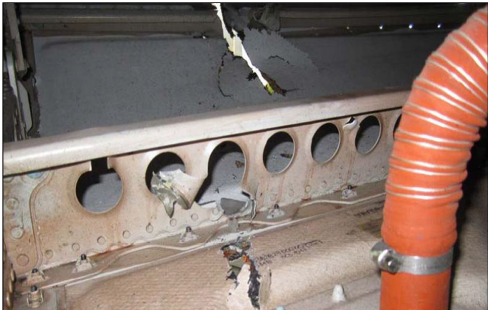
Figure B36: Stringer 5 LH impact damage
