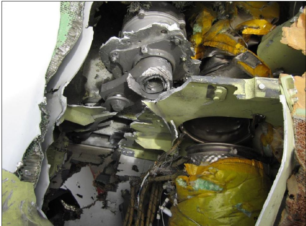
Figure B30: Damage to the drive motor located at leading edge Drive Rib No. 4
