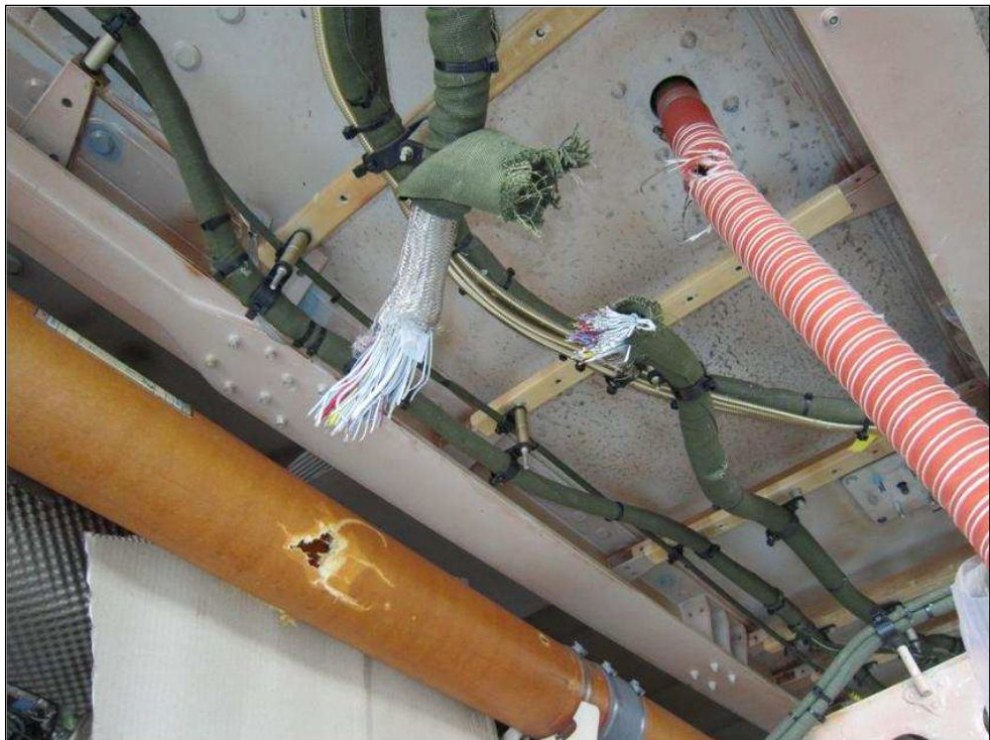
Figure B47: Wiring harnesses within the belly region of the aircraft structure were damaged from the liberated engine debris. Shown is harness 1525VB (route 1MK). All wires were severed
