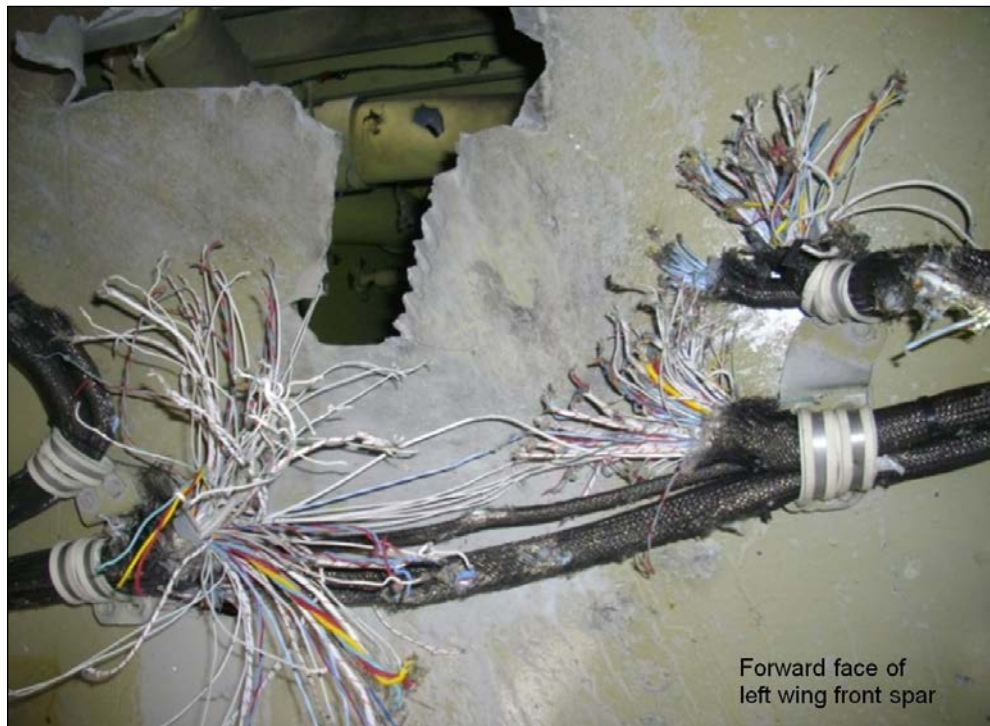
Figure 10: Damage to wiring in the belly fairing
