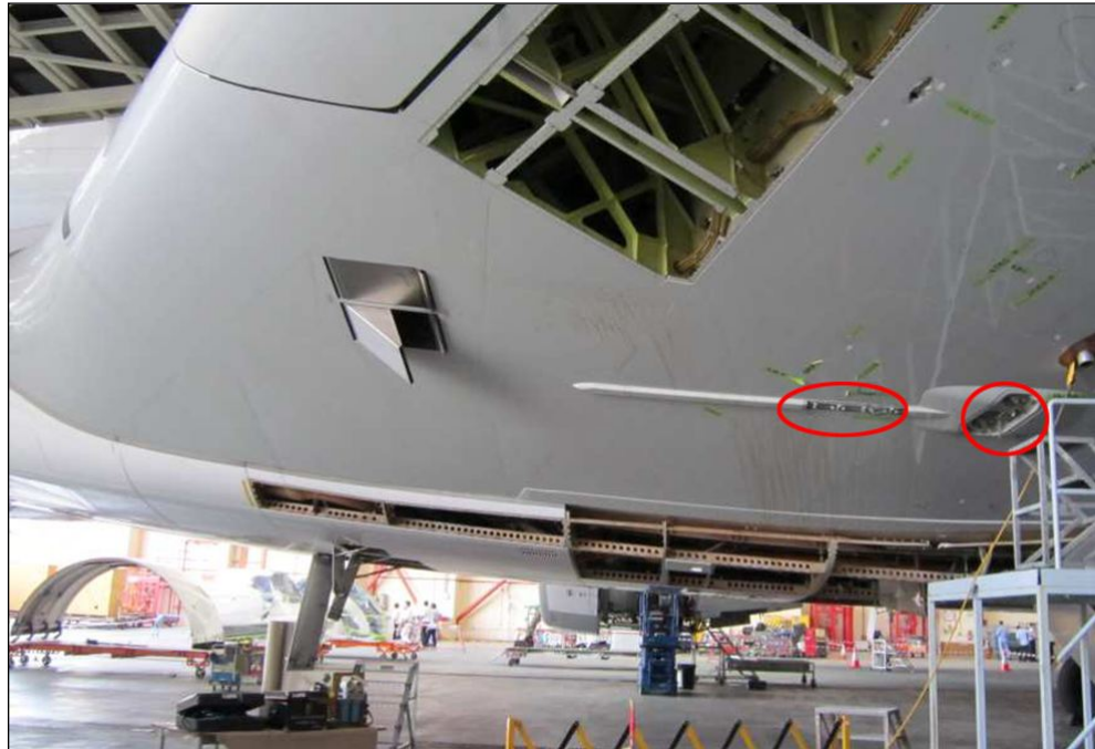
Figure B51: Damage to the 1M harness that supplied to the left wing forward fuel pump
