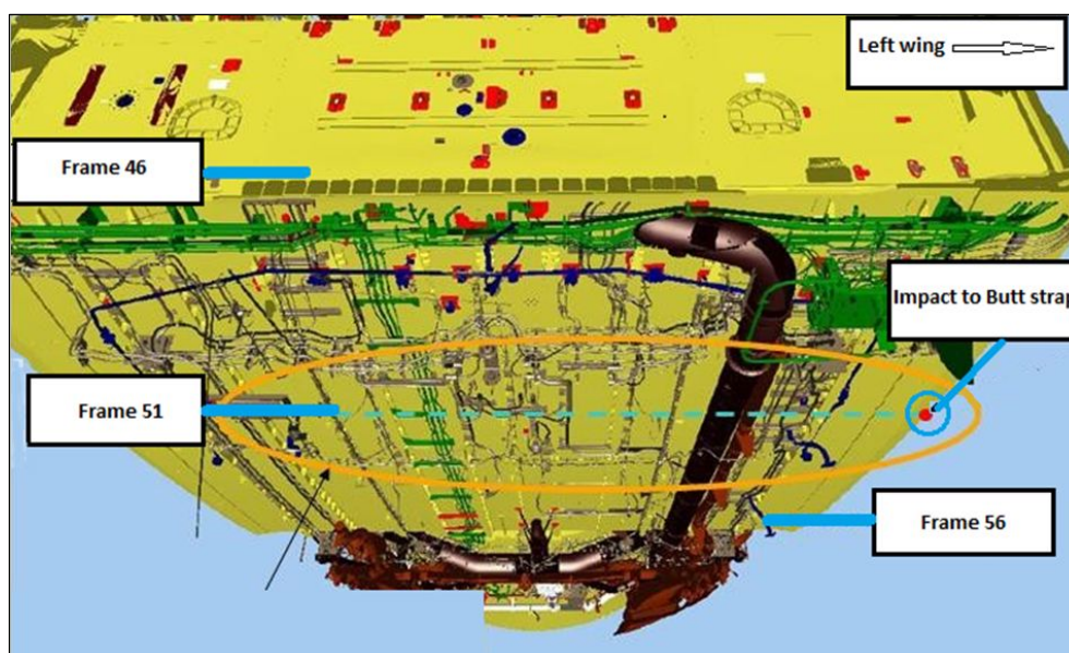
Figure B23: Schematic of the butt-straps damage between Frame 52 and 51
