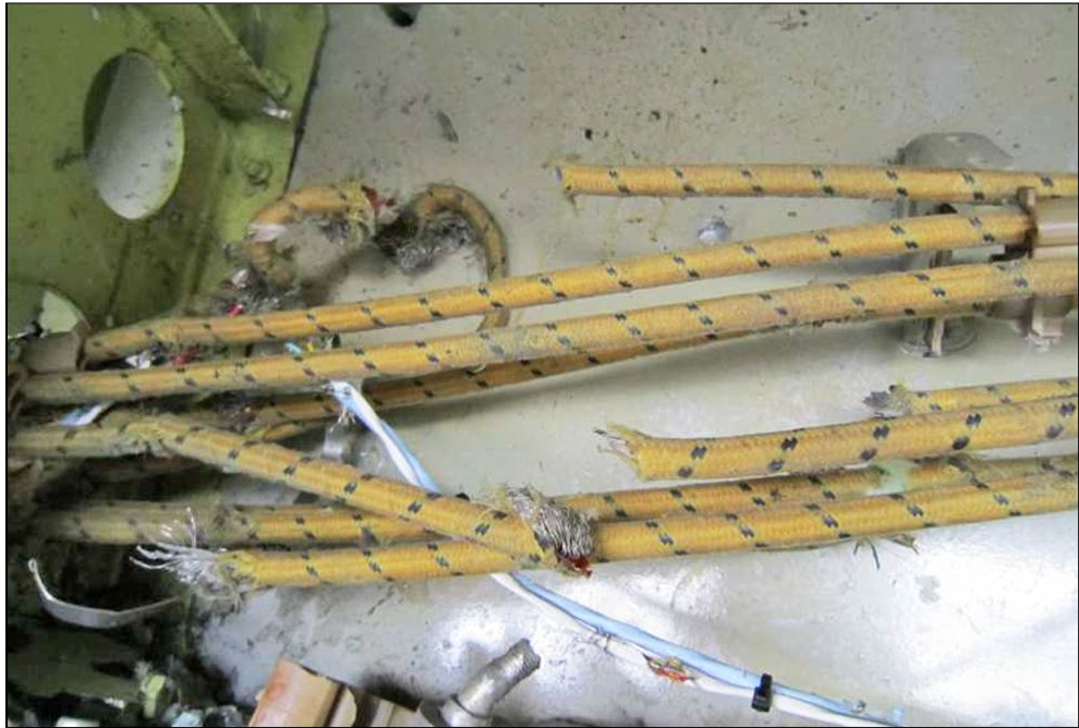
Figure B47: Wiring harnesses within the belly region of the aircraft structure were damaged from the liberated engine debris. Shown is harness 1525VB (route 1MK). All wires were severed
