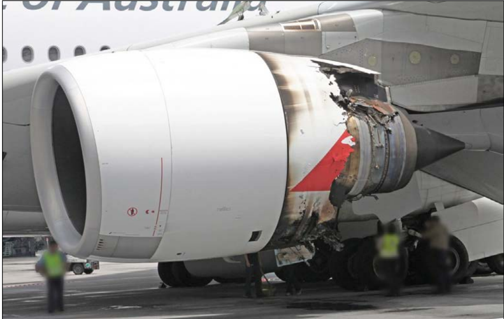
Figure 5: General damage to the No. 2 engine
