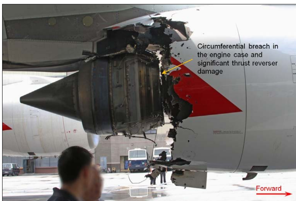
Figure 32: General damage to the engine (looking outboard)
