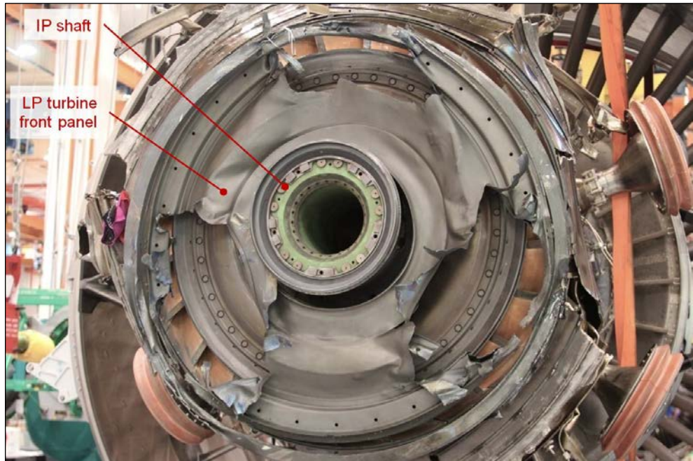
Figure 33: LP turbine front panel damage
