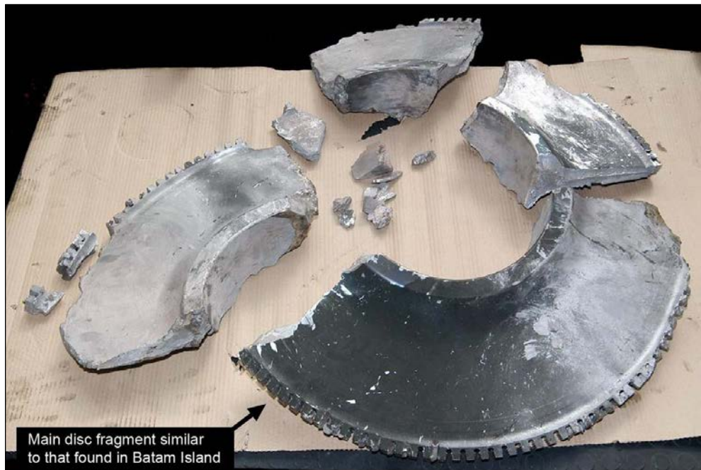
Figure 48: Trent 900 IP turbine disc after overspeed burst test
