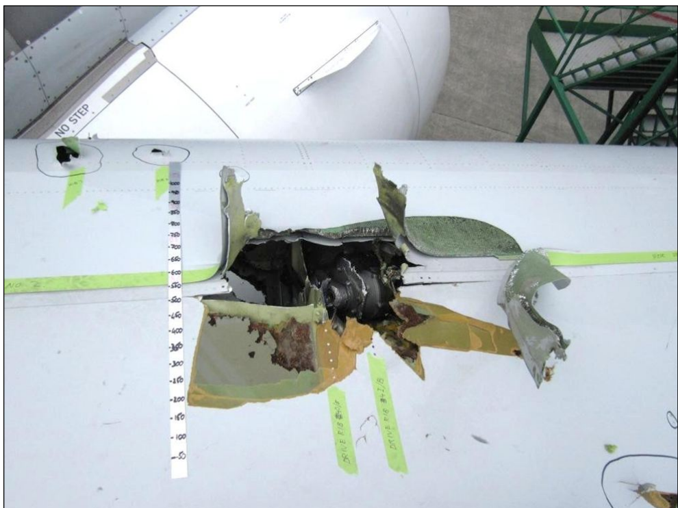
Figure B30: Damage to the drive motor located at leading edge Drive Rib No. 4
