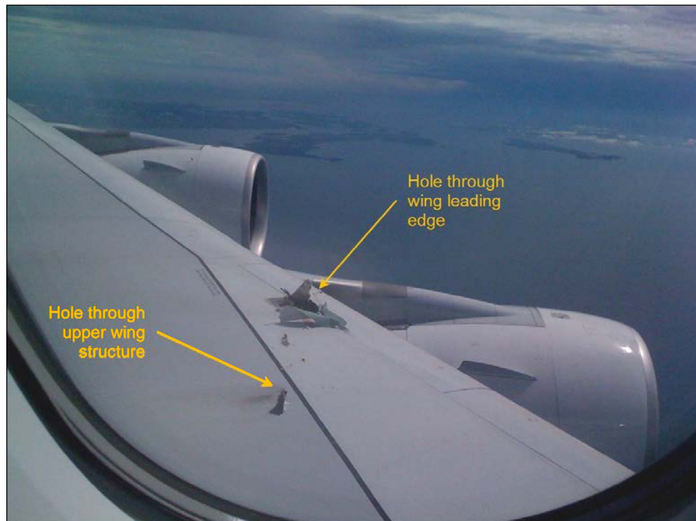
Figure 7: Examples of damage to the left wing
