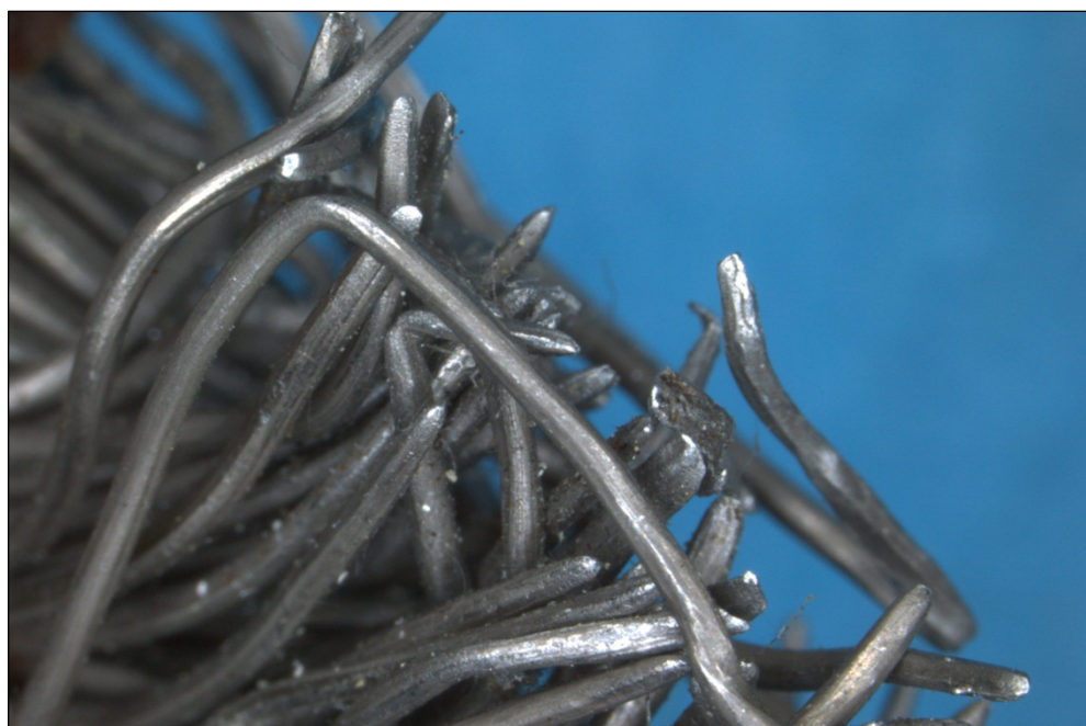
Figure D10: Magnified view of the severed end of VFG2 wiring
