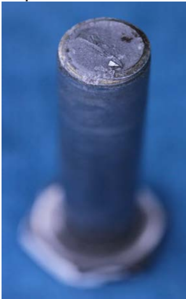
Figure 2: Failed lower torque link attachment bolt
