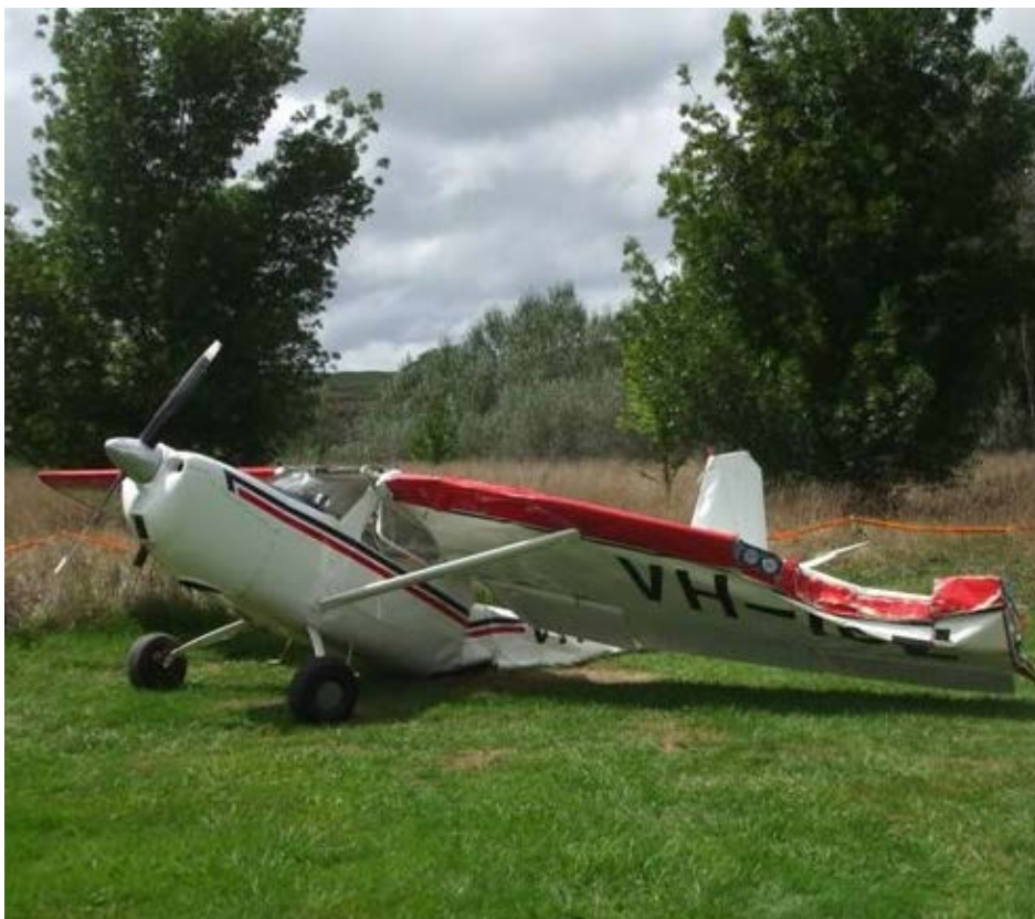
Figure 2: VH-ICE damage to the left wing
