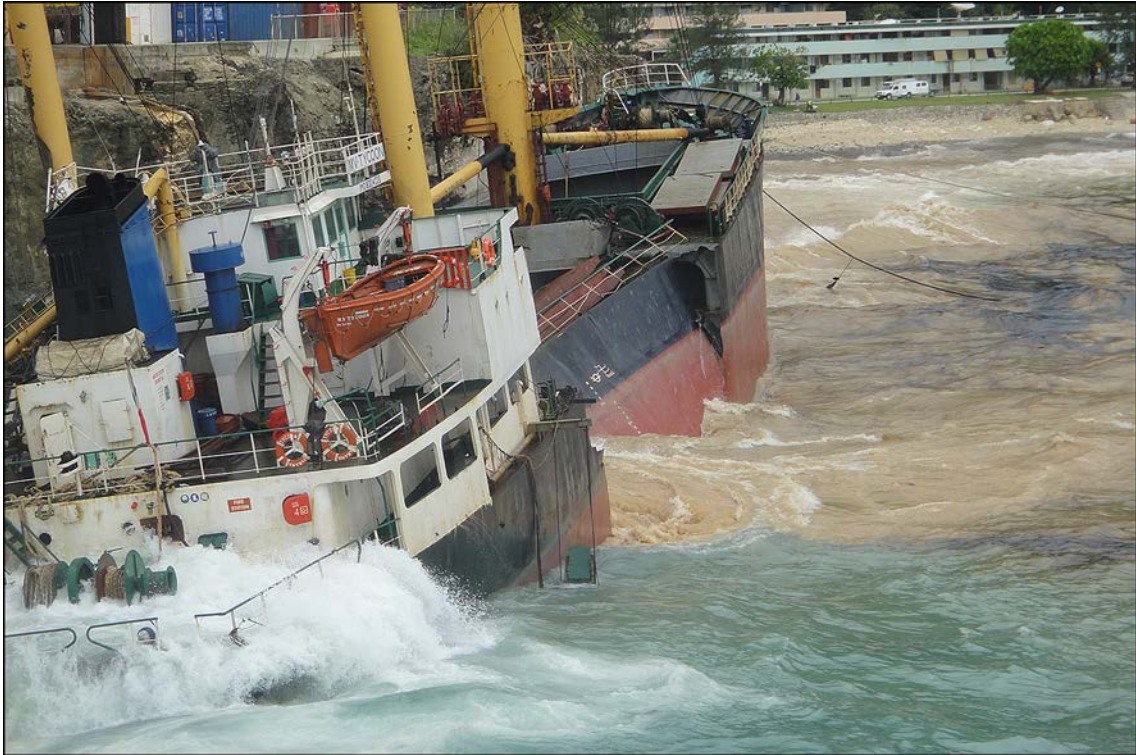
Figure 7: Failure of the ship's hull at number 2 hold
