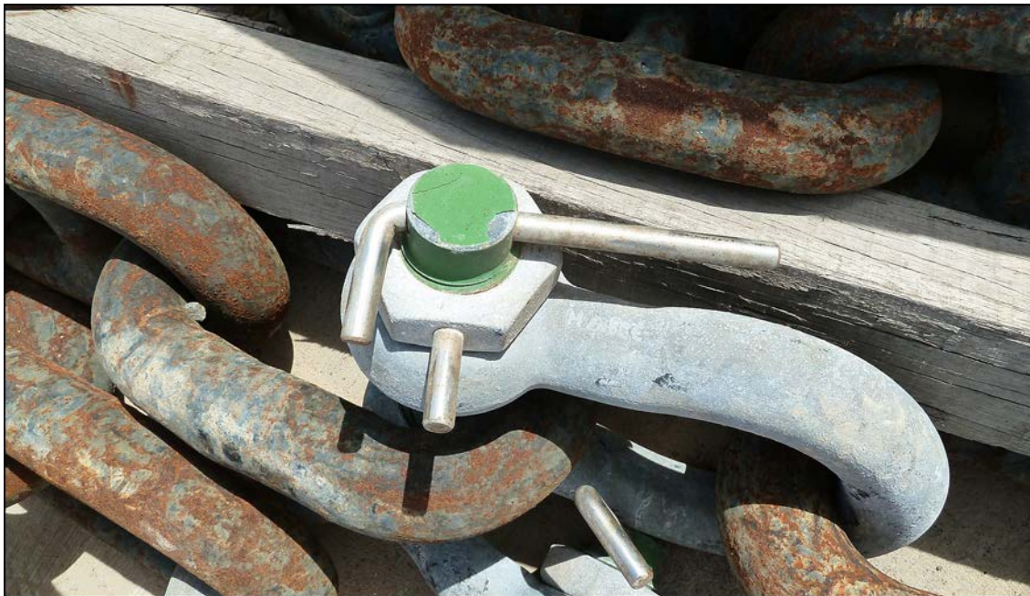
Figure 16: A new joining shackle with the improved 'locking pin' arrangement
