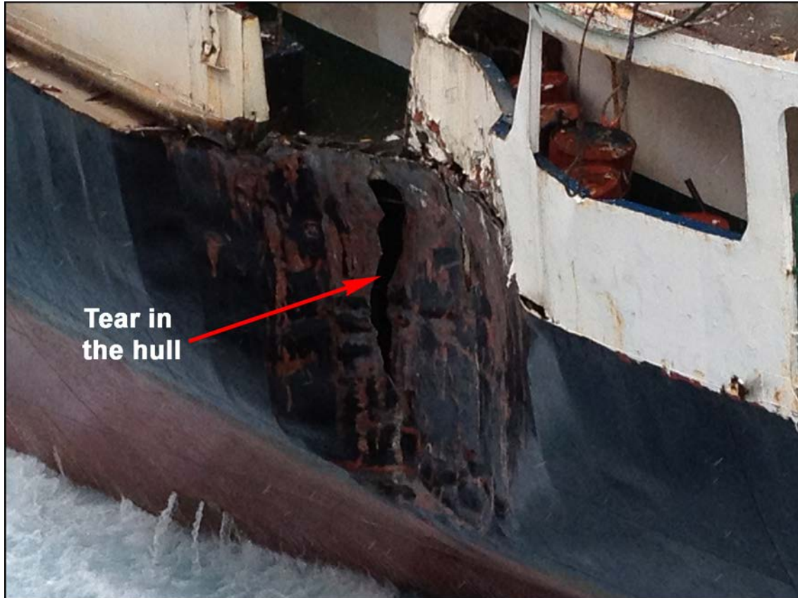
Figure 5: Tear in the hull in way of the engine room
