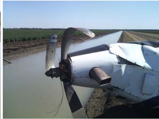
Power line wrapped around propeller
