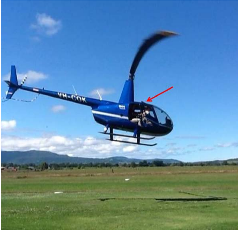
Figure 2: Pilot's door (arrowed) open as helicopter turned left
