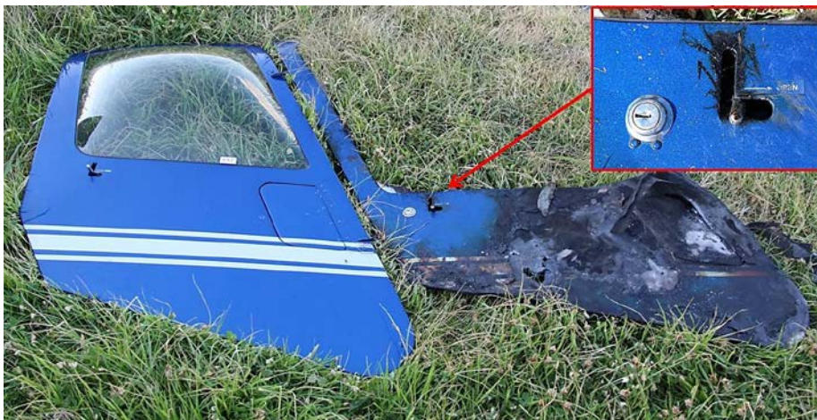
Figure 15: Rear right door alongside pilot’s door (burnt) as noted on-site. Note the position of the external door handle
