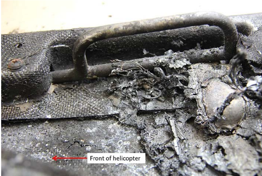
Figure 14: Pilot’s door internal handle position as noted post-accident
