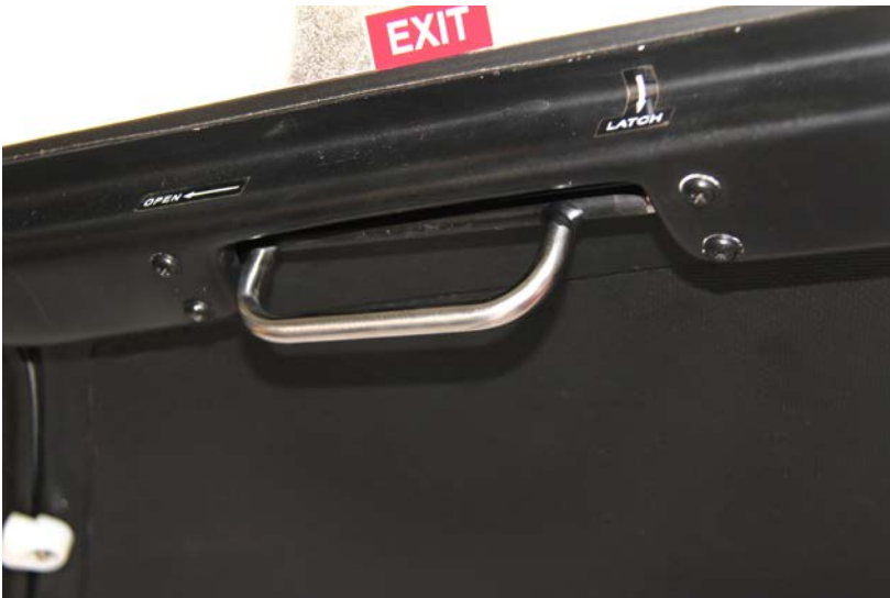
Figure 7: Exemplar R44 pilot's door from the inside showing the looped handle in the unlatched (fully forward) position
