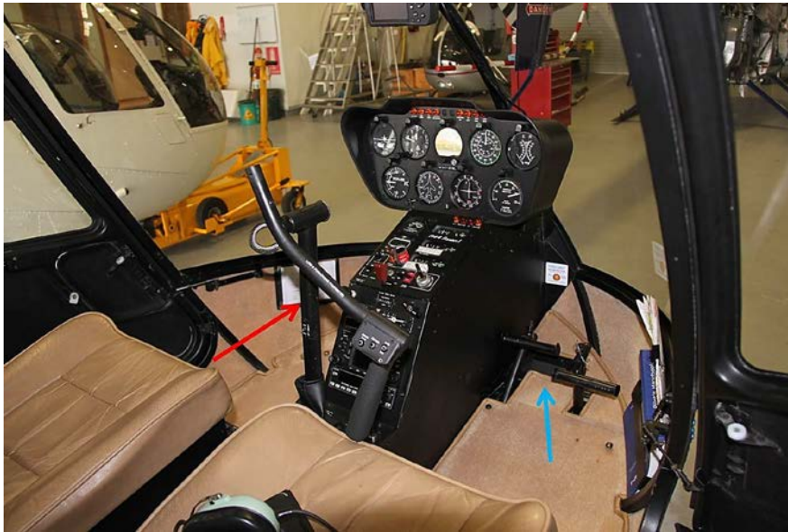
Figure 8: Exemplar R44 cockpit flight controls showing the cyclic column (red arrow) and right grip and the tail rotor pedals (blue arrow)
