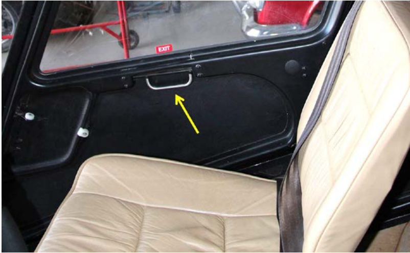
Figure 6: Exemplar R44 pilot's door from the inside showing the looped operating handle fully to the rear and rotated to the down and latched position
