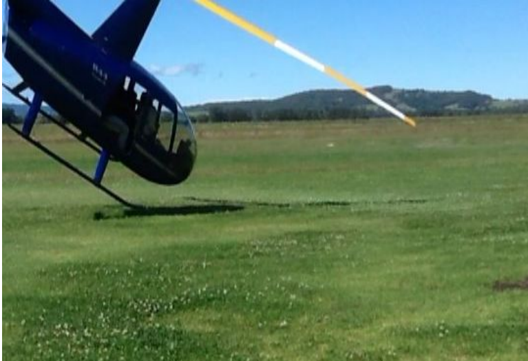
Figure 4: Helicopter pitched nose-down with the front of the right skid contacting the ground. Note pilot’s door closed in toward the fuselage
