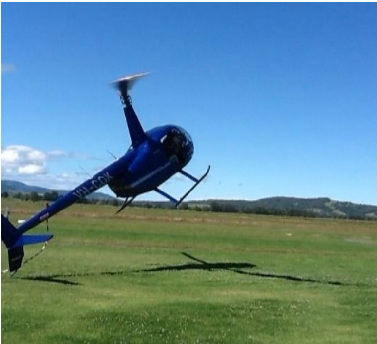
Figure 3: Helicopter pitched up with the tail skid contacting the ground
