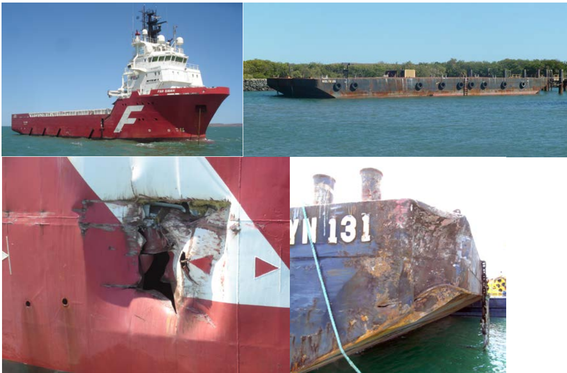
Collision between the Singapore registered offshore supply vessel Far Swan and the barge Miclyn 131 at Dampier, Western Australia on 6 October 2010 (ATSB investigation MO-2010-006).
