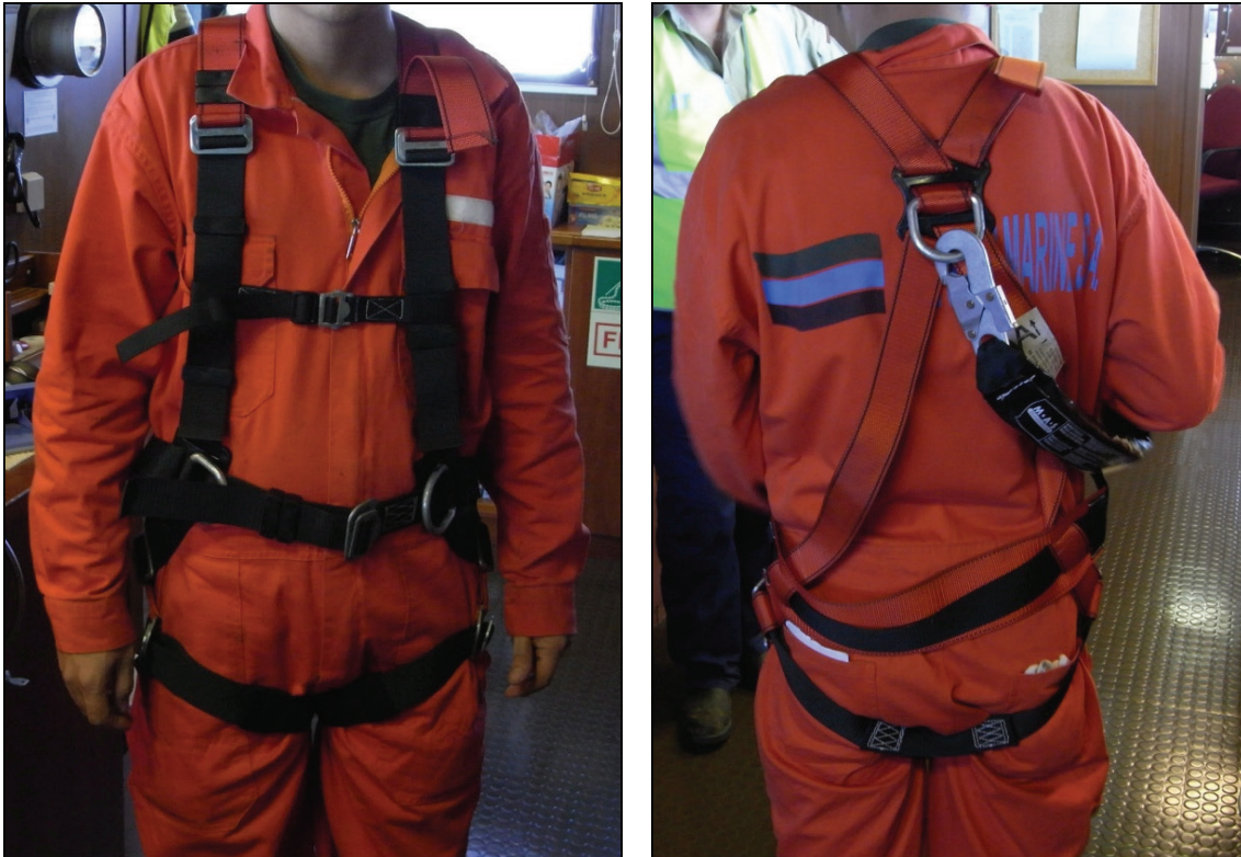
Figure 3: The same type of safety harness as used on 17 November (front and back)
