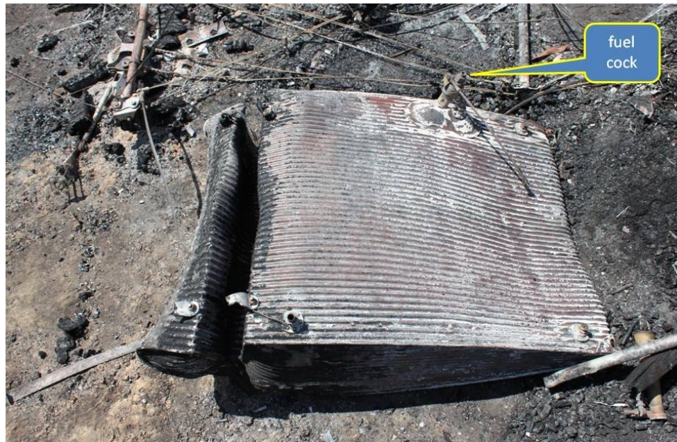
Figure 1: Main fuel tank (inverted) and fuel cock
