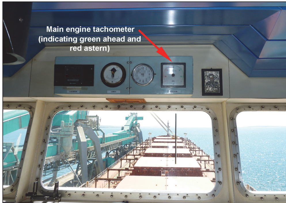
Figure 15: Main engine tachometer mounted on the bridge front
