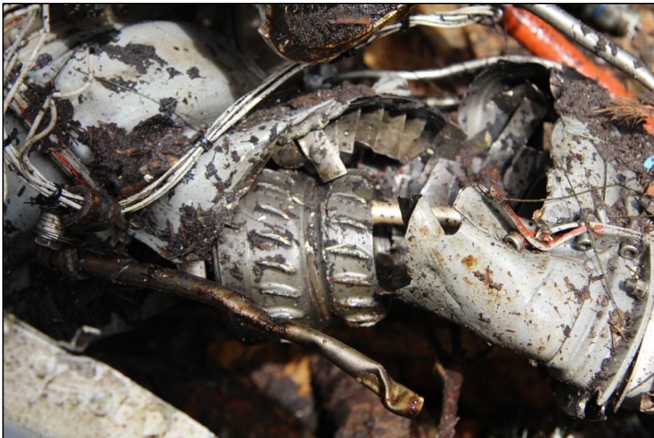
Figure 6: Sheared axial compressor blades
