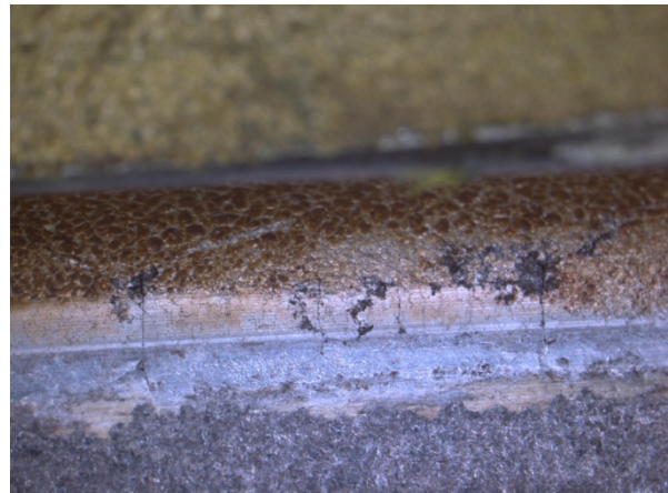
Figure 5: Axial cracks adjacent to the peened radius
