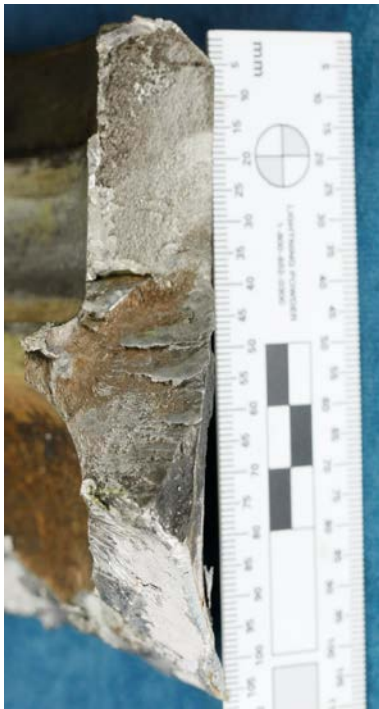
Figure 3: Discoloured and grey fracture zones
