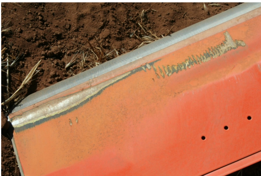
Main rotor blade witness mark tip damage (Investigation AO-2008-078)
