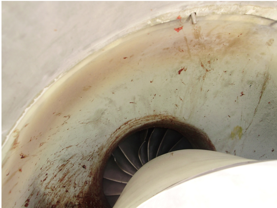
Metroliner turboprop engine ingestion following birdstrike with multiple galahs
