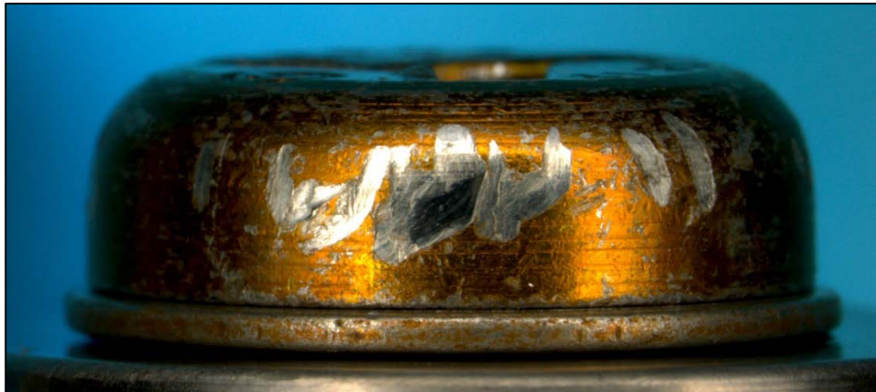
Figure 18: Typical contact marks left by masked multi-grip-type hand tools
