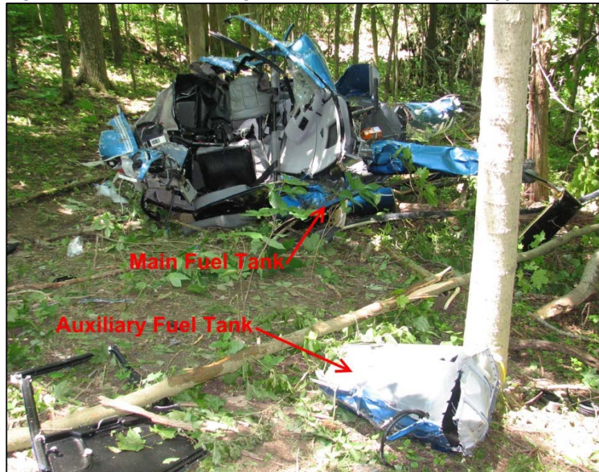
Figure 7: Accident involving an R44 fitted with bladder-type fuel tanks
