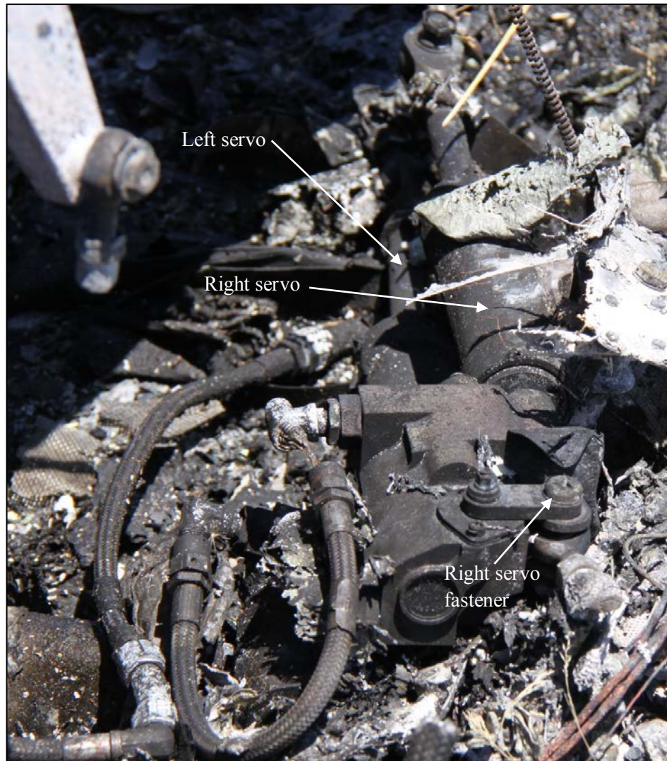
Figure 13: Right-front, left-front and exemplar hydraulic-boost servos
