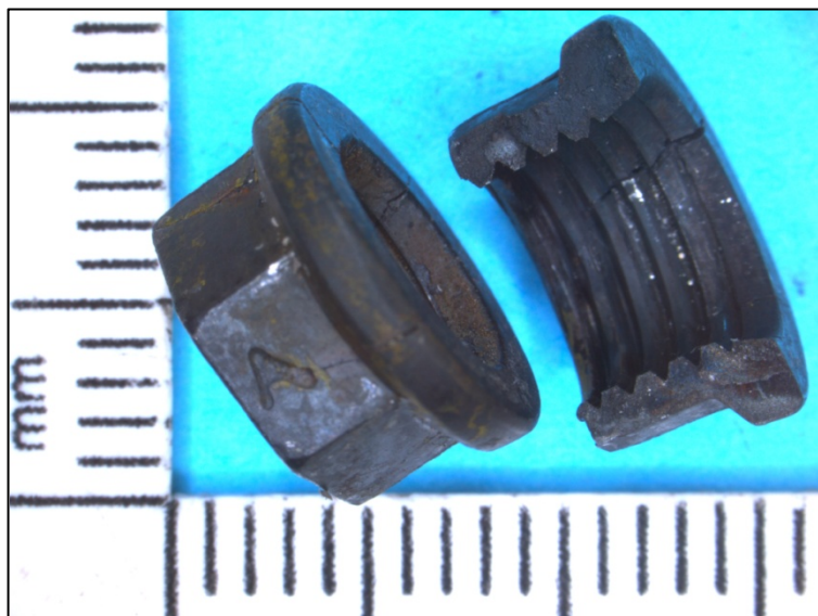
Figure 15: Cracked self-locking nuts
