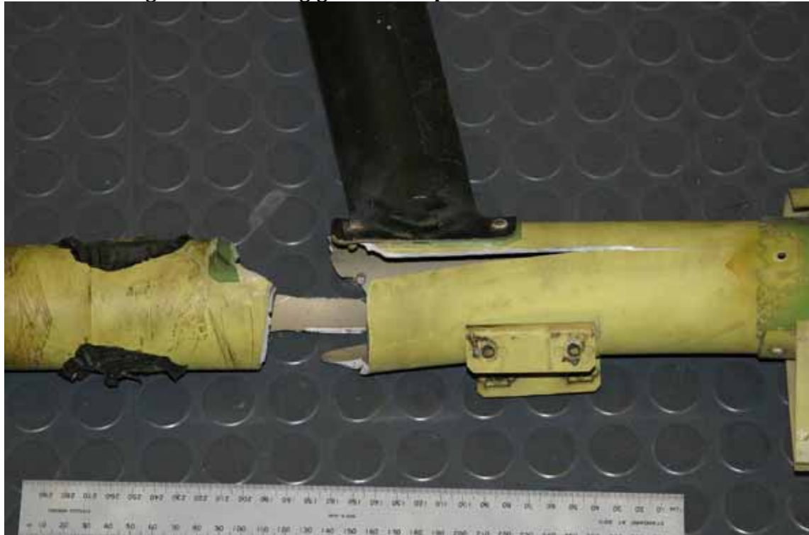
FIGURE 2: Right front landing gear strut – point of fracture
