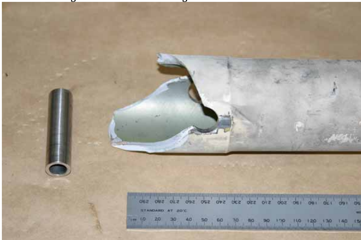
FIGURE 9: Drag brace connection bushing and fractured rear strut
