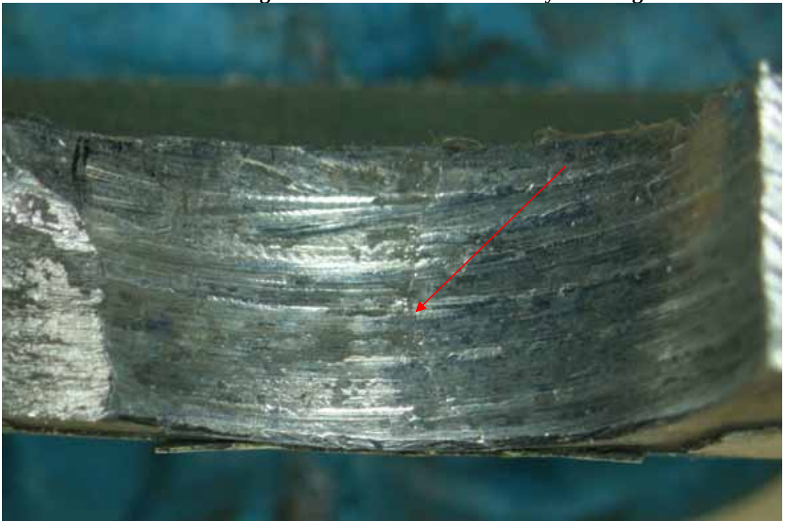
FIGURE 6: Bore of the drag brace hole with the secondary cracking indicated
