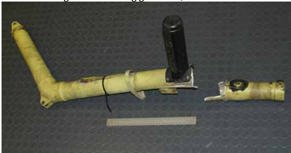
FIGURE 1: Right front landing gear strut, as received
