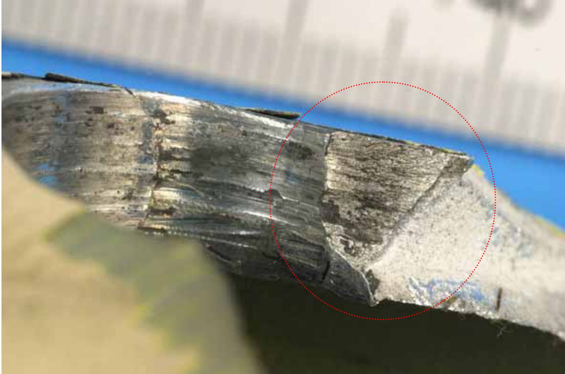
FIGURE 5: Closer view of the pre-existing cracking (circled)
