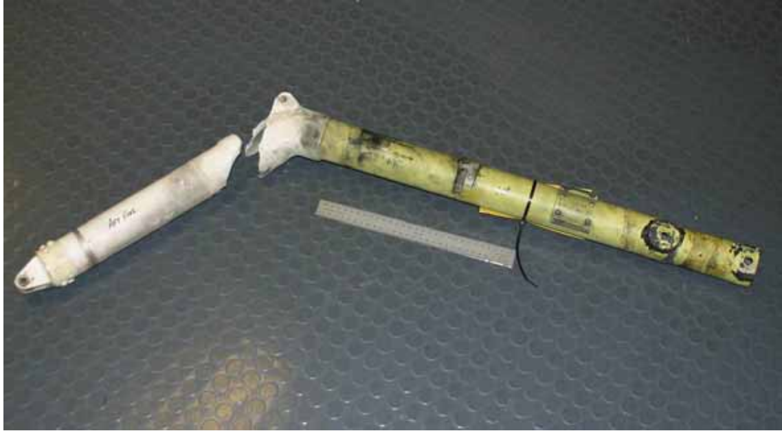
FIGURE 3: Right rear landing gear strut, as received
