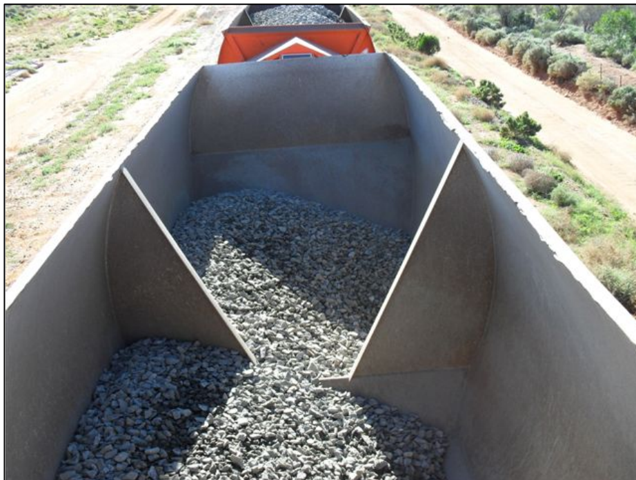
Figure1: Wagon AHBY0001R post derailment showing uneven load
