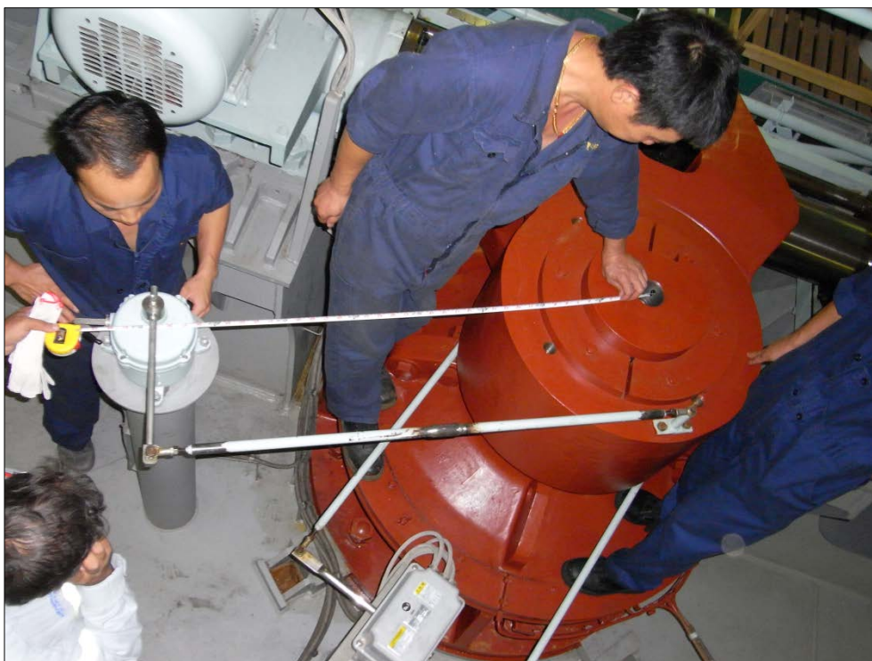
Figure 14: Ship's engineers checking the transmitter/rudder stock dimension
