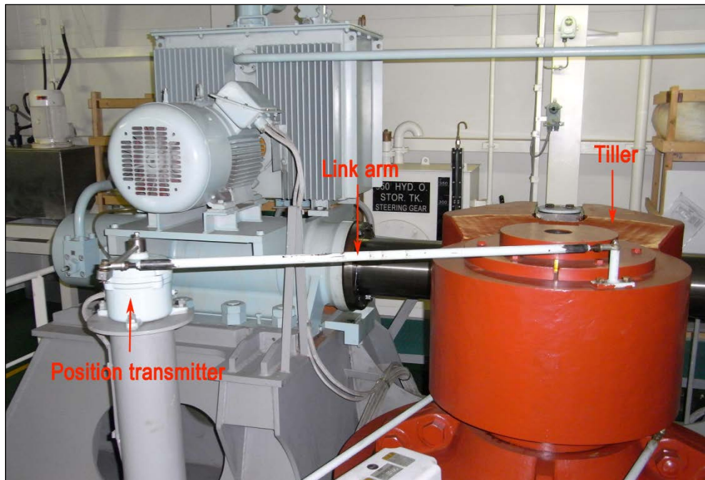
Figure 9: Rudder position transmitter link arm
