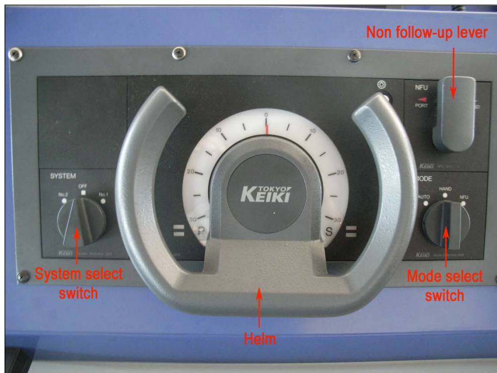
Figure 5: Steering control stand
