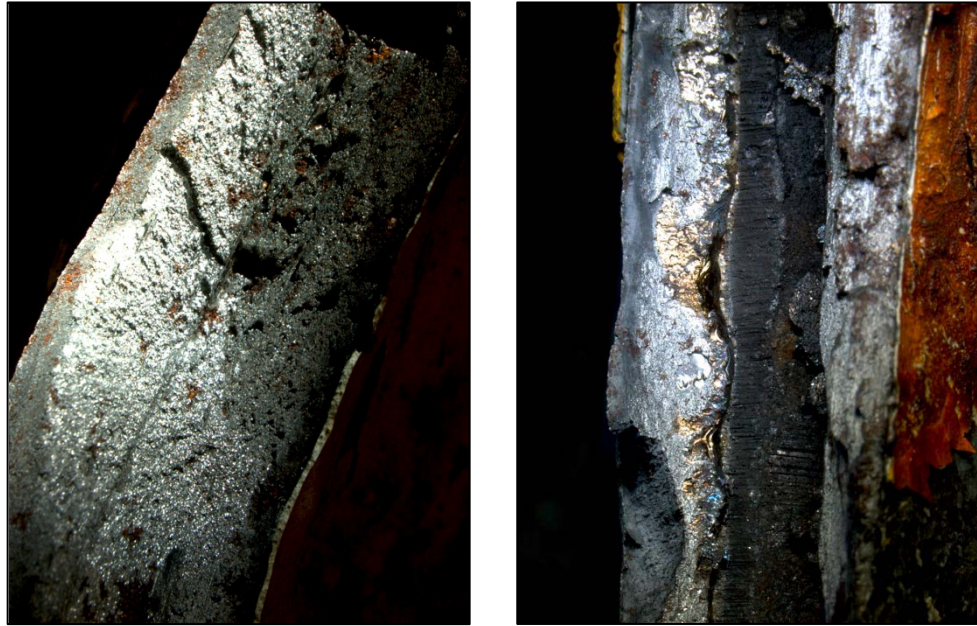
Figure A7a & b: Crystalline (bright) and overload (grey) fractures in the left photo; lack-of-fusion (gold) and lack-of-penetration (dark grey striations) areas are in the right photo
