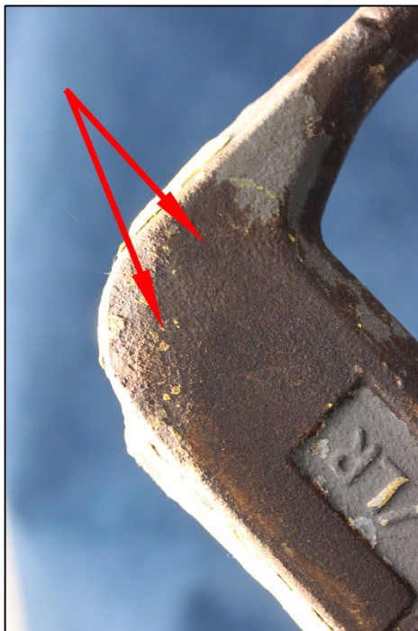
Figure A5a & b: Flat (arrowed) on the port/forward corner of the top plate and witness mark/paint (arrowed) on the port/forward corner of the twistlock's underside
