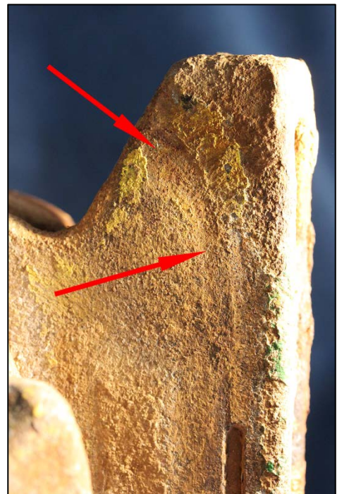
Figure A5a & b: Flat (arrowed) on the port/forward corner of the top plate and witness mark/paint (arrowed) on the port/forward corner of the twistlock's underside
