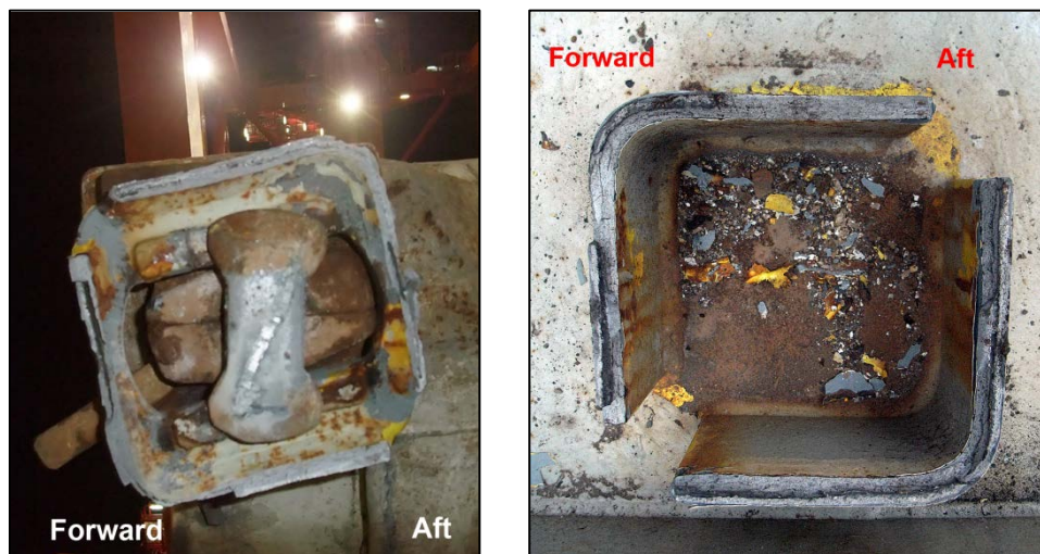
Figure A1a & b: Twistlock assembly and top plate, as made fast to the container, and the two side plates, as made fast to the hatch cover.
