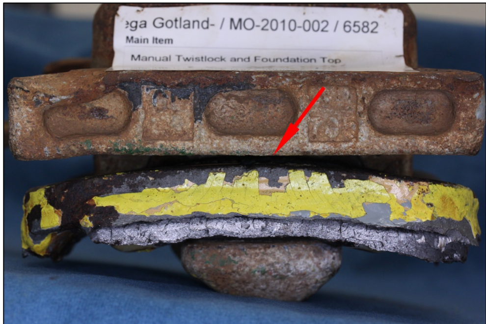
Figure A3a & b: Deformed foundation top plate with two indentations on the underside (arrowed)
