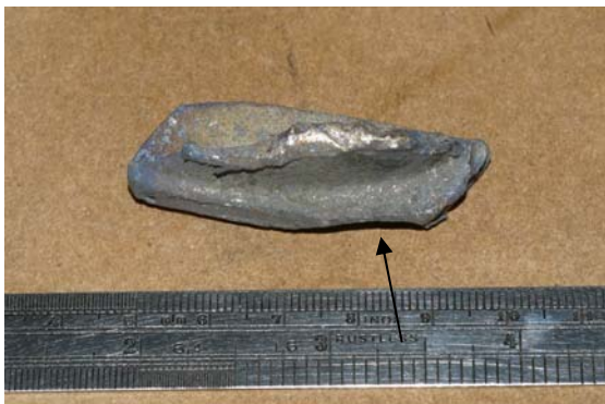
Fig. 10 HPC first-stage blade stub, showing missing forward corner (arrowed).
