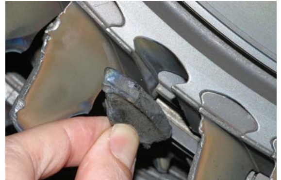
Fig. 9 Orientation of the blade stub with respect to the HPC first-stage disk.
