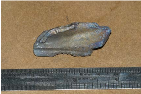
Fig. 8 HPC first-stage blade stub as-recovered.
