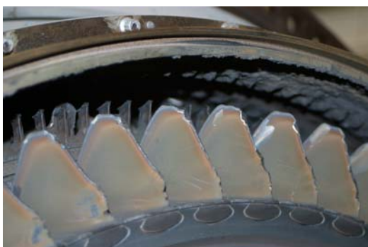
Fig. 2 (Top L) Module 41 assembly as examined. First-stage high-pressure compressor disk is at the left.
