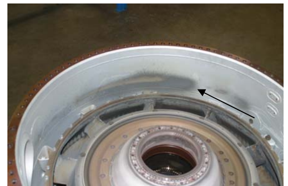
Fig. 14 (Top L) Module 33 intermediate case looking forward. Evidence of forward gas flow and combustion.
