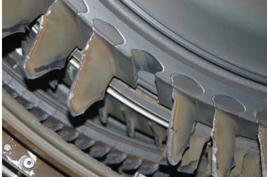
Fig. 6 HPC 1 disk with missing blade.
