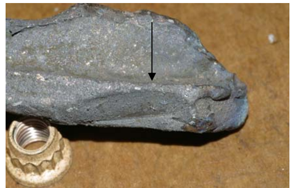
Fig. 11 HPC first-stage blade stub corner fracture with suspected fatigue crack initiation region shown.
