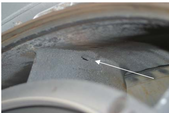
Fig. 14 (Top L) Module 33 intermediate case looking forward. Evidence of forward gas flow and combustion.
