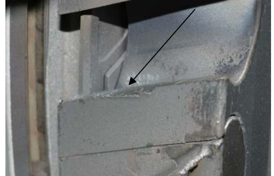
Fig. 7 Metal deformation and burring found on the slot edge.
