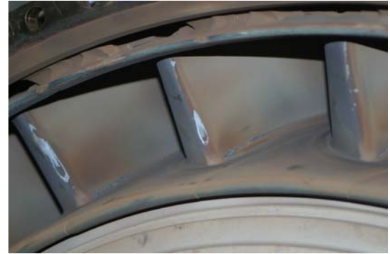
Fig. 13 Minor damage to the leading edges of the IP turbine inlet guide vanes.
