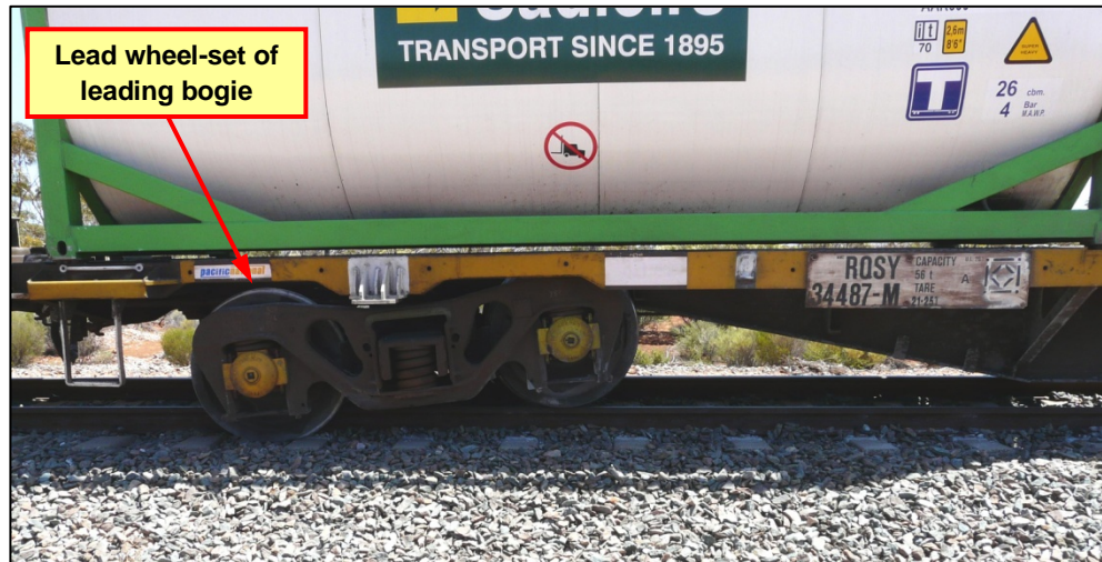
Figure 9: First of derailed wagons RQSY34487-M, note the lead wheel-set of the leading bogie
