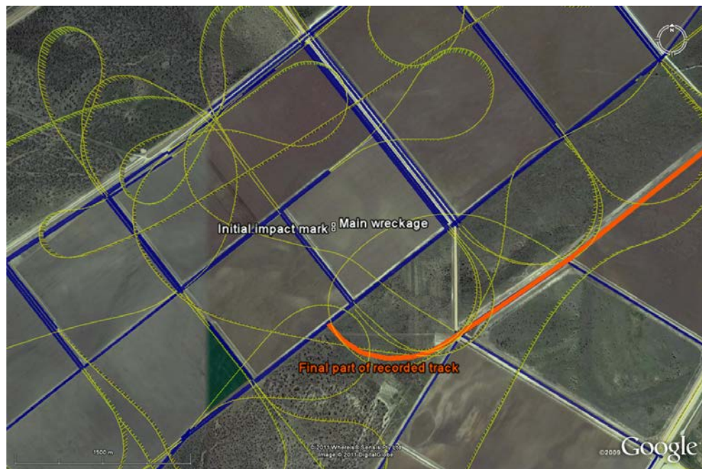
Figure 4: Accident site overview showing the recorded aircraft track (yellow), spray runs (blue) and the final part of the recorded track (orange)
