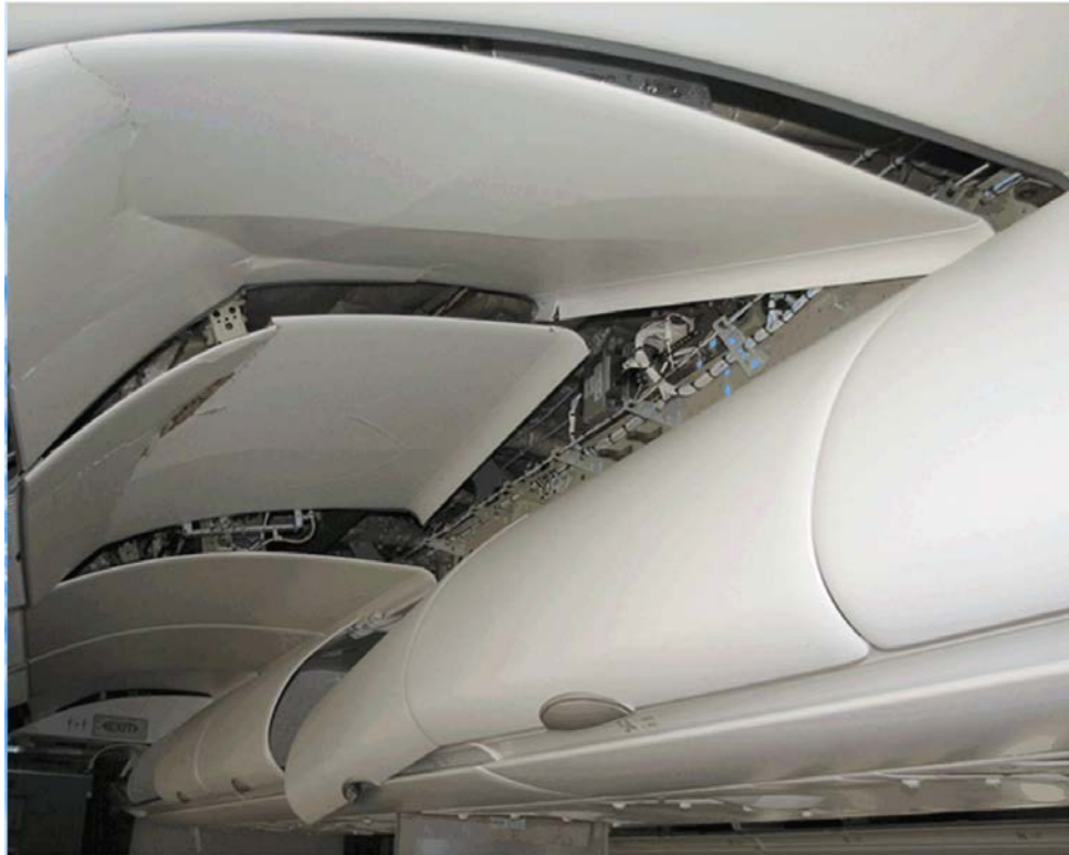
Damage to overhead cabin panels after an in-flight upset, Airbus A330 (VH-QPA) Western Australia (AO-2008-070)
