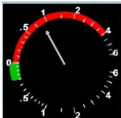
Figure 4: Illustration only of VSI with TCAS lights
