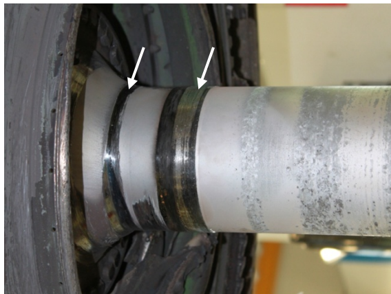
Figure 9: LP turbine shaft showing evidence of contact with IP shaft
