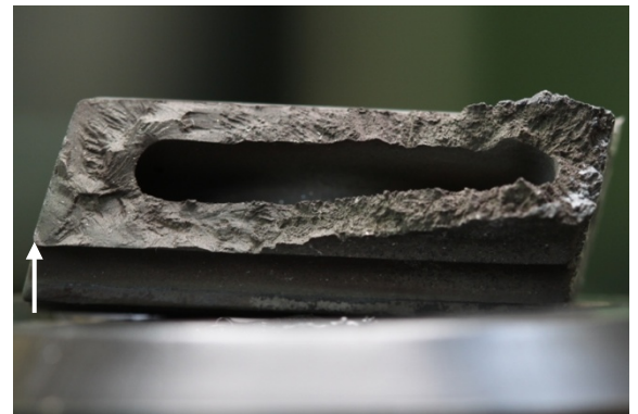
Figure 9: LP turbine shaft showing evidence of contact with IP shaft
