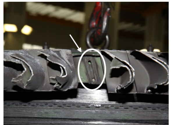
Figure 11: Stage-2 LP turbine blade root. Fatigue crack origin arrowed
