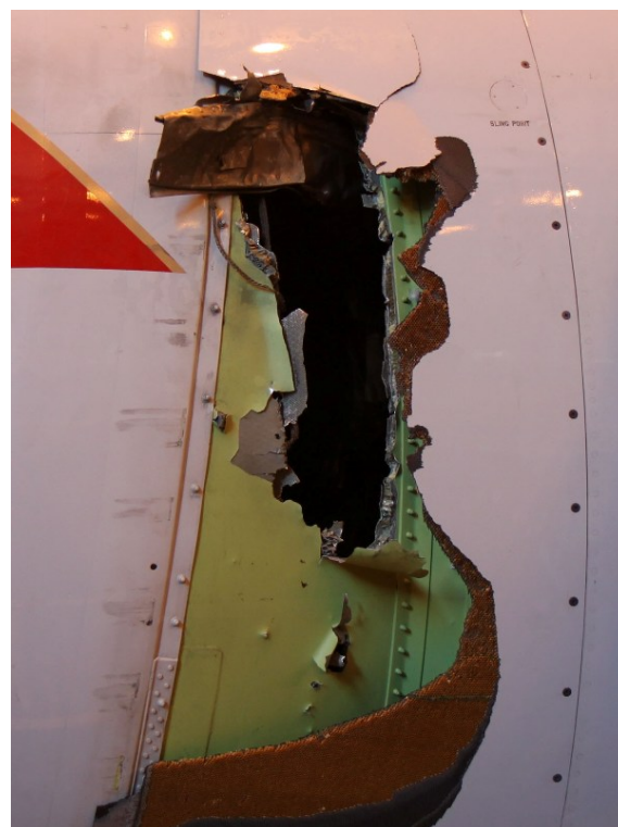
Figure 2: Perforation in the engine nacelle, right side
