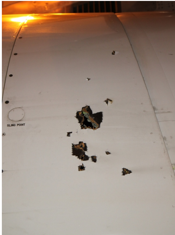
Figure 3: Punctures in nacelle, left side
