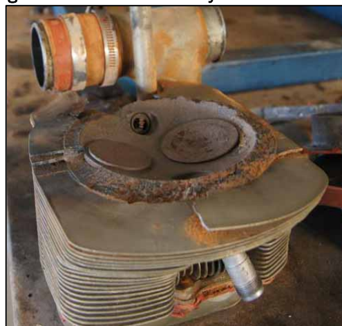
Figure 3: Failed number-4 cylinder
