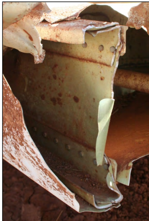
Figure 34: Rear spar inboard fracture
