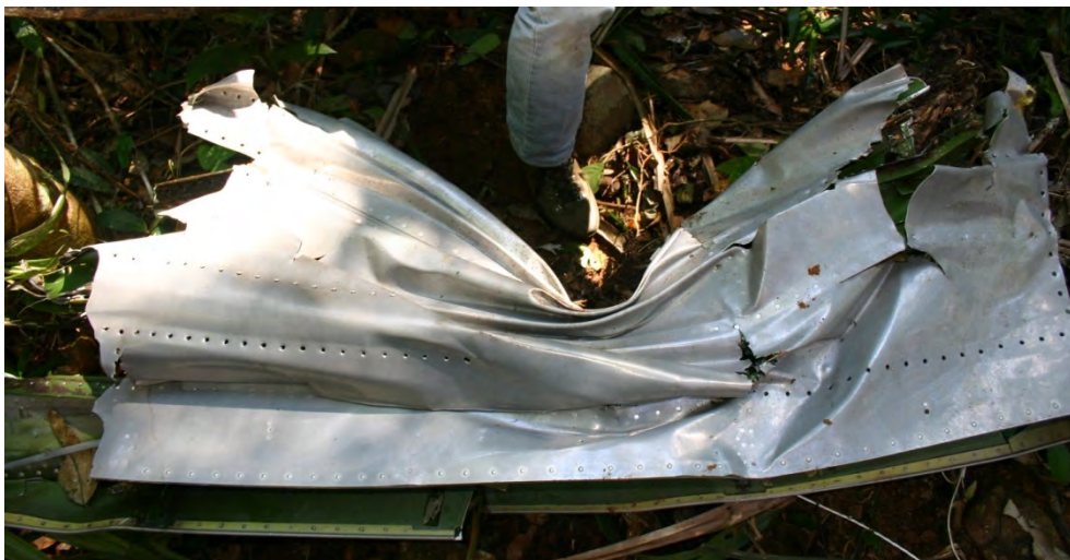
Figure 39: Partial penetration tree impact damage
