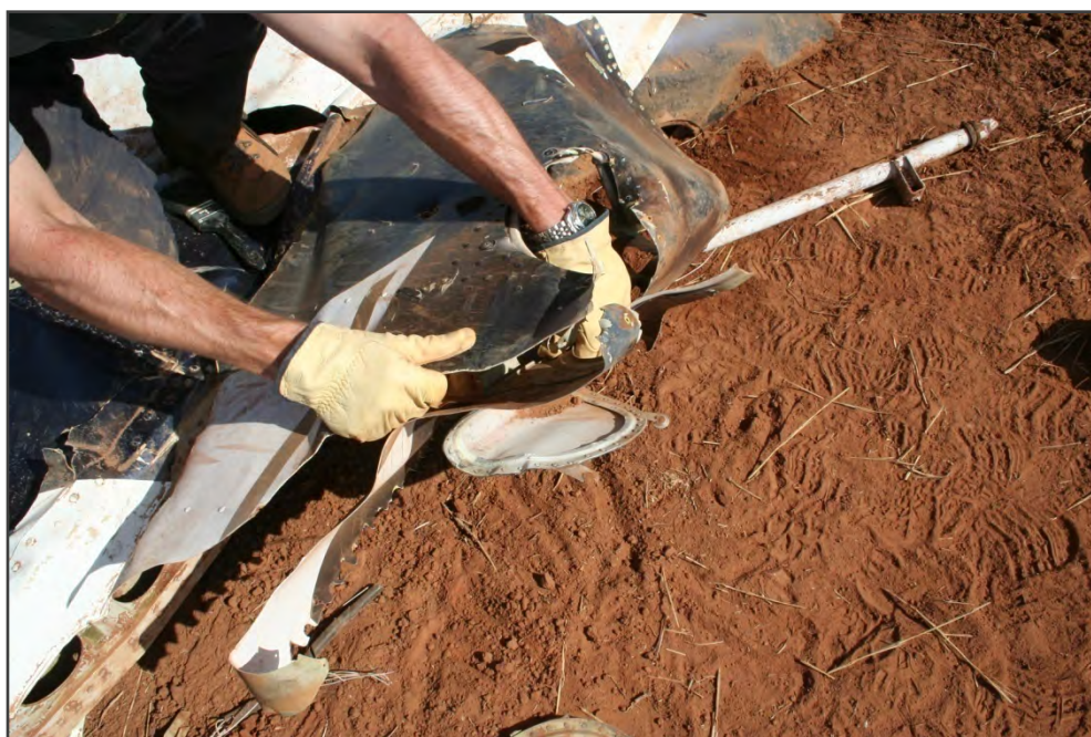
Figure 26: Leading edge deformation
