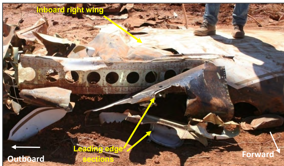
Figure 26: Leading edge deformation
