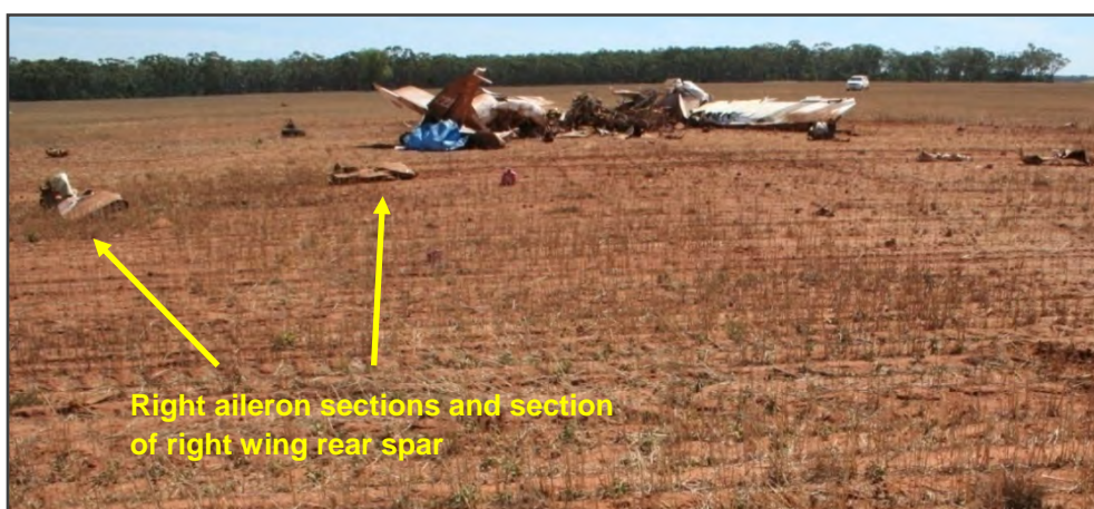
Figure 22: Right aileron pieces and section of the rear right spar
