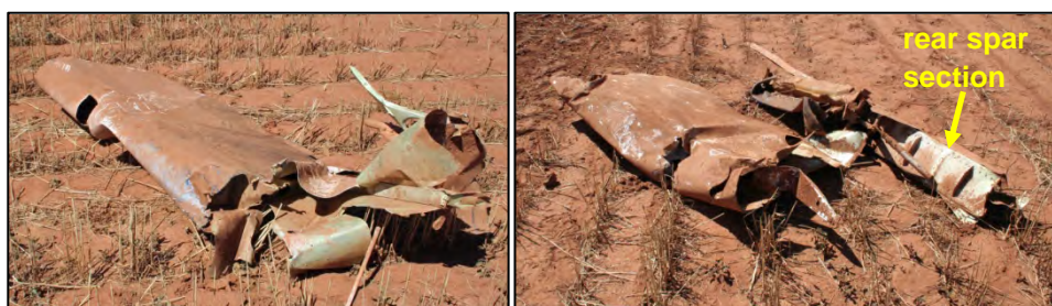
Figure 22: Right aileron pieces and section of the rear right spar
