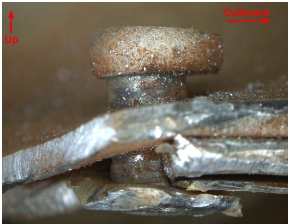
Figure B9: Elongated rivet from the main spar lower cap - adjacent to the fracture surface
