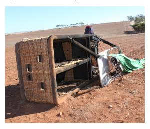
One of the burners was damaged during the landing sequence. After some minor repairs, a functional test was carried out on both burners with no evidence of any defects or anomalies. There was LPG in each of the five on-board storage cylinders with a calculated total quantity of 215 L. Each burner was connected to a cylinder that was at least 60% full at impact.
