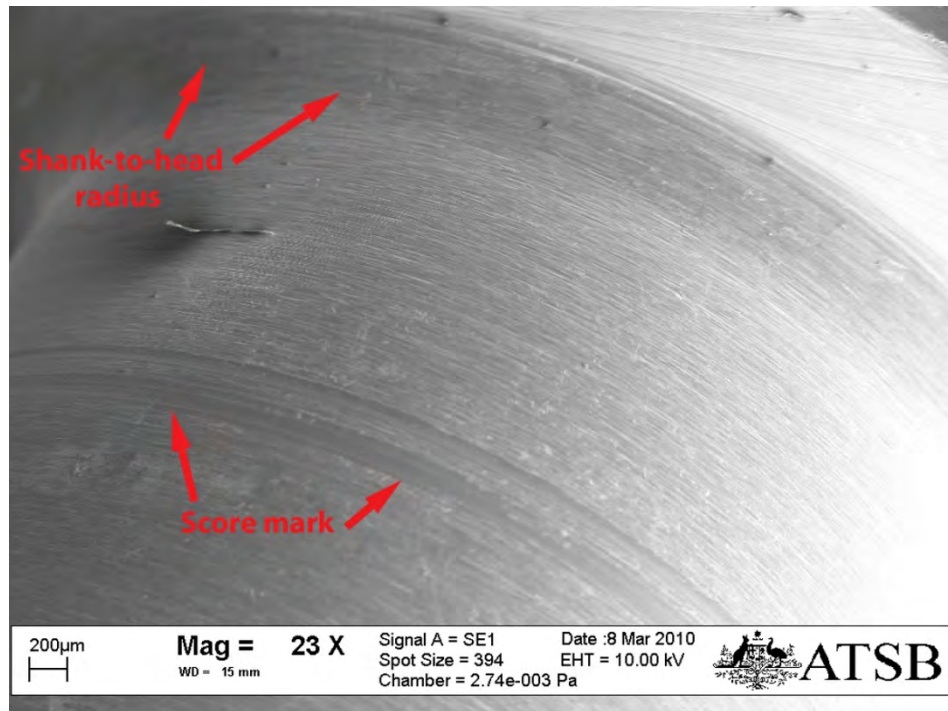
Figure A14: Low magnification scanning electron microscope image showing the shank-to-head radius of Bolt R. Note the smooth appearance of the radius, and the machining marks observed on the radius and the under-head bearing surface
