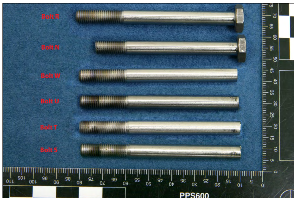
Figure A9: Carrier bolts following disassembly of the first stage reduction carrier. Note that Bolts S, T, U and W failed under the bolt head, Bolt N failed through the threaded section, while Bolt R remained intact
