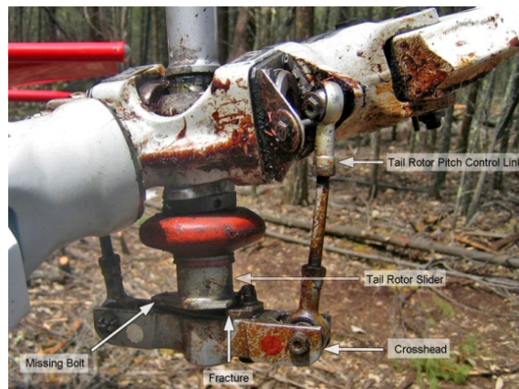
Figure 4: Slider and crosshead
