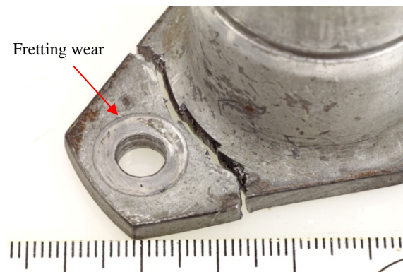
Figure 7: Fretting wear on slider flange
