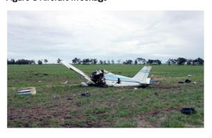
All of the aircraft's primary structure and flight controls were located at the accident site and there was no evidence of fire (Figure 3) or pre-
