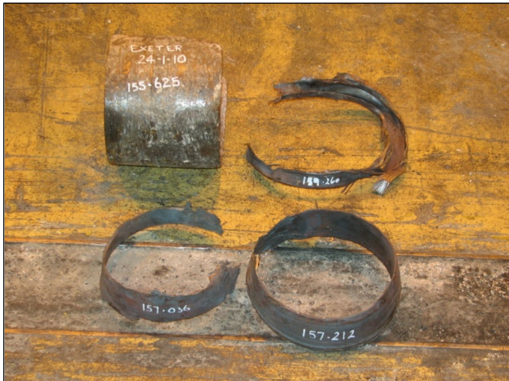
Figure 4: Remains of R3 bearing
