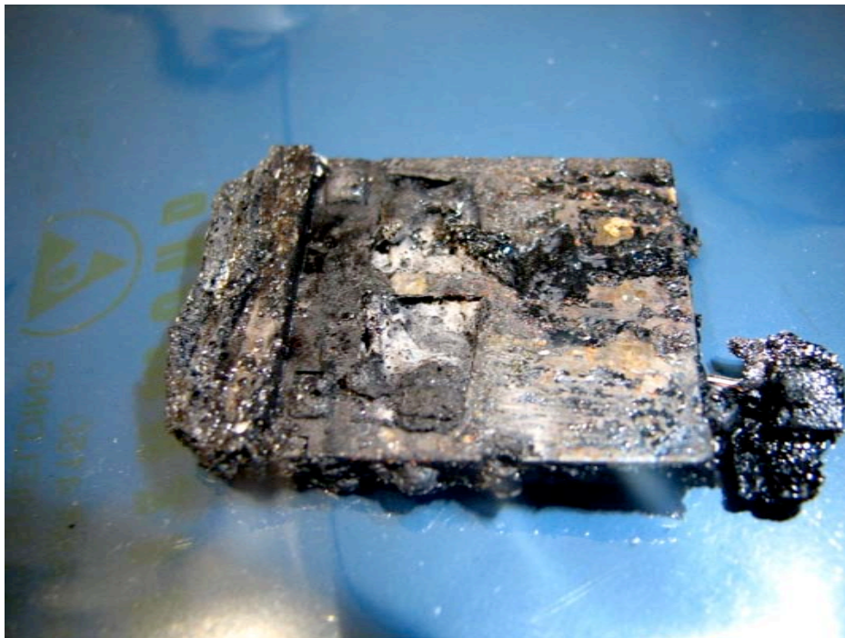
Figure 5: SD/MMC enclosed in its socket (reverse)
