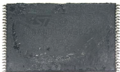
Figure 15: NAND device after inspection and cleaning
