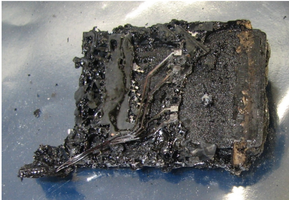
Figure 5: SD/MMC enclosed in its socket (reverse)
