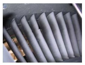
**Fig. 7** Impact damage to the engine outlet guide vanes.
