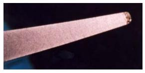
**Fig. 29 (Above)** Low-magnification view of the early stages of the fatigue cracking – vague arrest marks evident radiating out from the blade edge.
