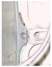
**Fig. 17** Elongation of the nose cowl mounting flange bolt holes.
