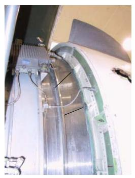
**Fig. 16** Location of several nose cowl bolts fractured during the blade separation event.
