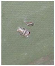
**Fig. 18** Nose cowl bolt head and washer embedded into the underside of the right fan cowl.
