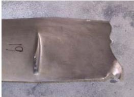
**Fig. 4 (Top L).** Damage to the contact surfaces of the fan part-span shrouds.
