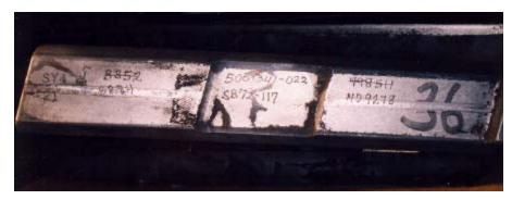
Fig. 23 Blade identification on the root face
