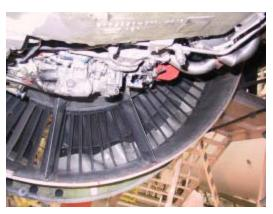
**Fig. 8** Lifting of a section of the bypass duct lining in front of the outlet guide vanes.
