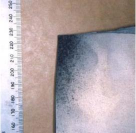
**Figs. 20 & 21 (Top)** Blade dove-tail root surfaces – free from significant galling and fretting damage and showing remnant dry lubricant.
