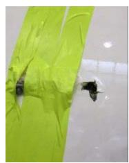
**Fig. 19** Small puncture in the right fan cowl caused by a fractured nose cowl bolt head.
