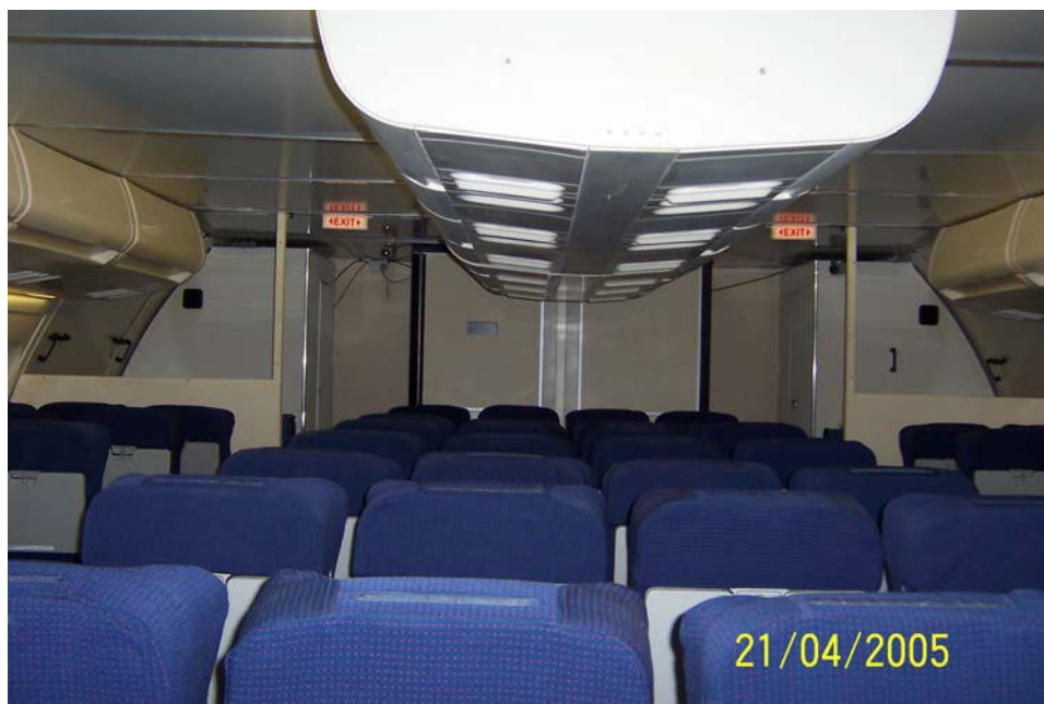
L6: Large Cabin Evacuation Simulator (LCES), upper deck view towards front of cabin, showing half-height bulkheads (photograph © Lauren Thomas 2005)
