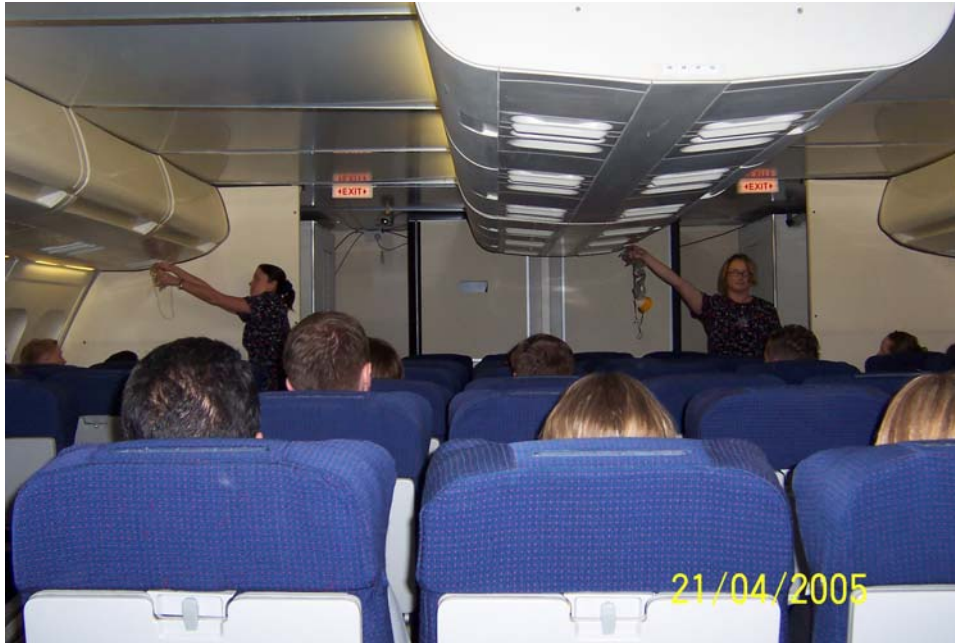
L9: Safety briefing in progress, Large Cabin Evacuation Simulator (LCES), showing full-height bulkheads (photograph © Lauren Thomas 2005)
