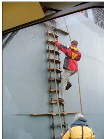
Figure 3: Pilot climbing the ladder, using manropes
