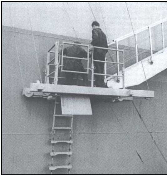
Figure 17: Welin Pilot Embarkation Platform System (PEPS)
