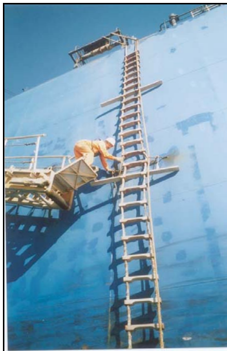
Figure 4: Rigging the pilot ladder
