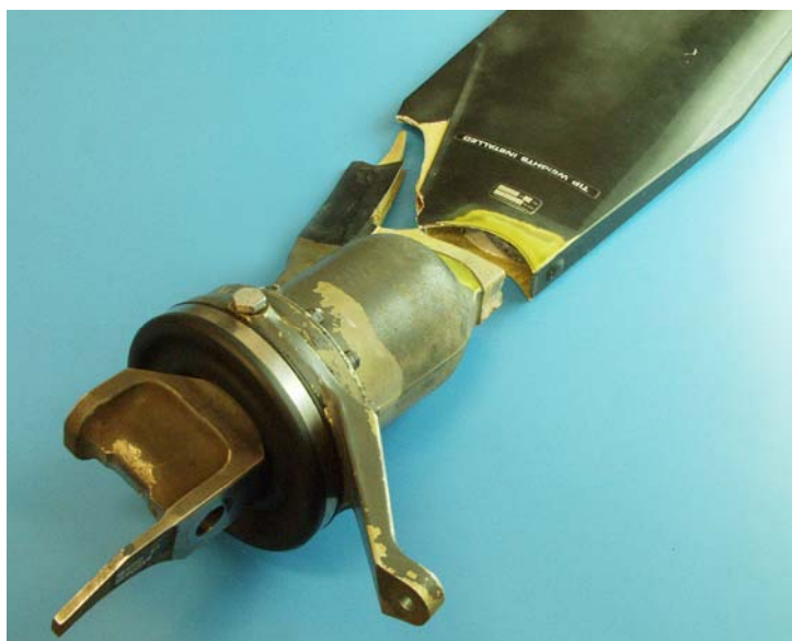
Figure 3: The fractured main rotor blade of VH-OHA
