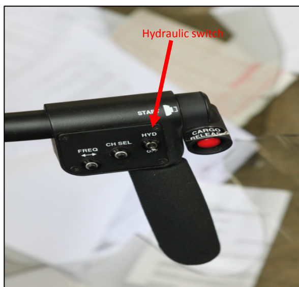
Figure 2: VH-ZVF Cyclic mounted hydraulic switch
