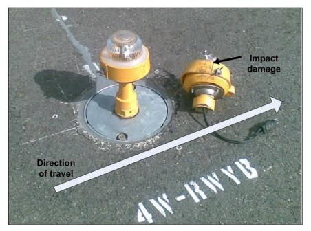
Figure 1: Damaged runway light with replacement (scrape marks indicated on the damaged light)
